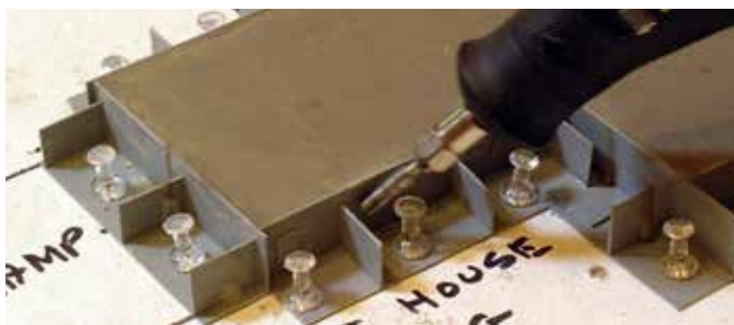
Fig. 12 Form vibration. Bruce used an empty mandrel mounted in a motor tool to vibrate the sides of the forms to release any air bubbles that might be trapped inside.
