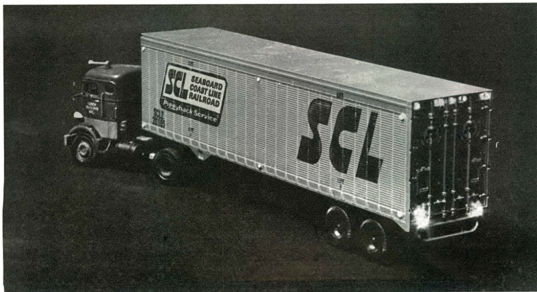
Fig. 7. This parked truck uses individual fibers run to a lamp located under the layout. If an Ulrich metal truck body were used, the lamp could be housed inside the vehicle, thus saving on the length of the fibers required. With lamp plus battery the truck could then be moved about.
