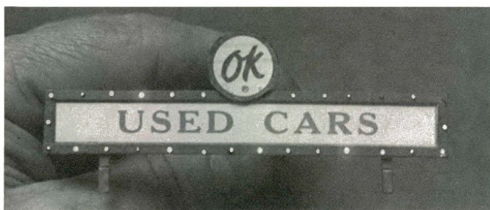
Fig. 6. Multistrand fibers make advertising signs like this one simple and cheap to illuminate.
