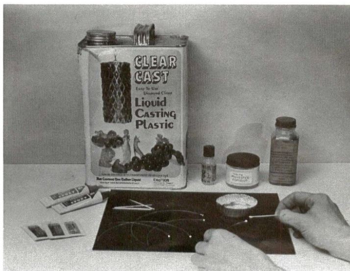
Fig. 10. Small lamp-shaped beads can be formed with epoxy or with polyester resin and pigment.
