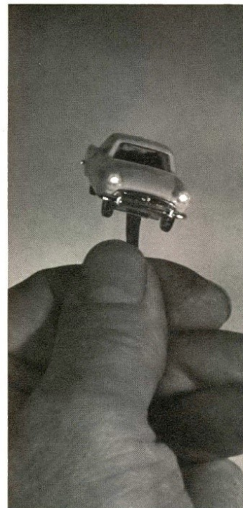
Fig. 4. Vehicle headlights throw a concentrated beam because of the fibers' directional quality.
