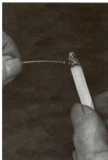
Fig. 9. Heat from a cigaret causes the end of a fiber to form a mushroom-shaped lens. Or, if you don't smoke, you can use a soldering iron.
