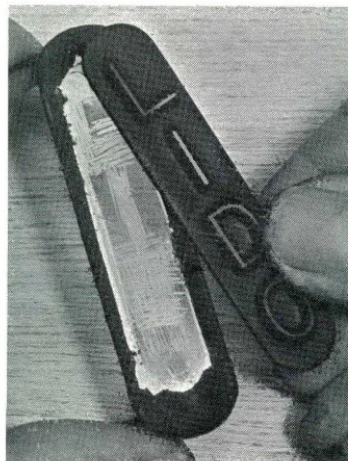
Fig. 19. The amount of scratching on the Plexiglas center piece controls the brightness of the vertical "neon" sign's letters.
