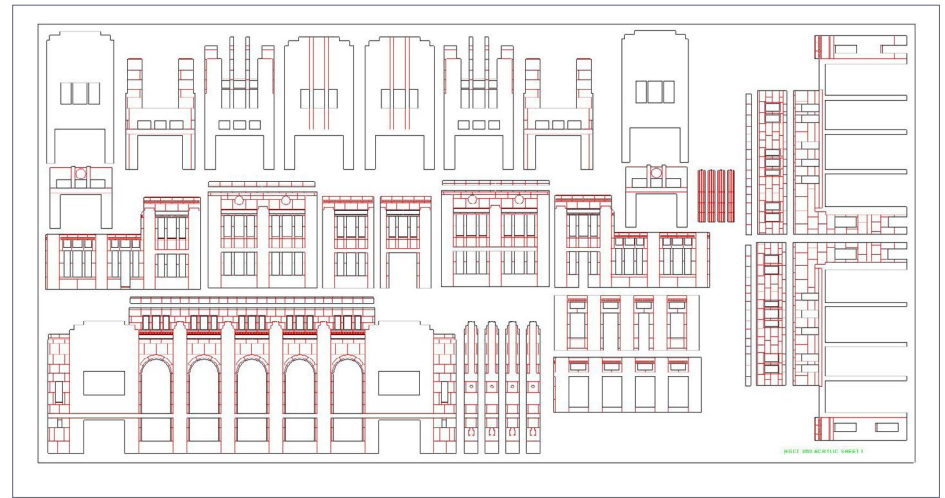
4. CAD drawing for laser-cutting on a 2' x 4' sheet of .060" acrylic. The red lines will be engraved into the sheet, the black lines will be cut through the sheet. With acrylic, attachment tabs are not necessary.
