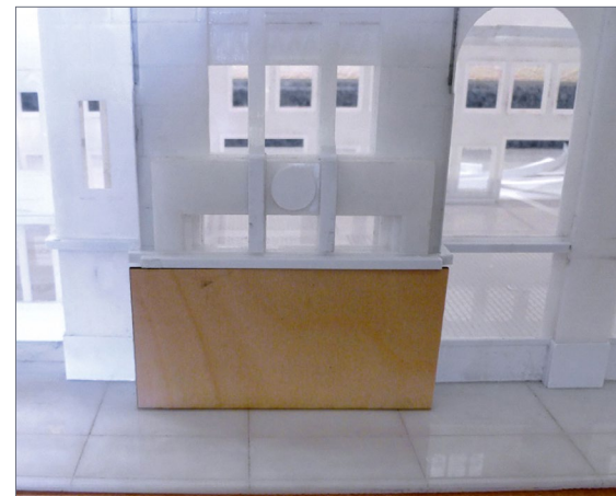
16. Installing the support strips for the front canopy.
