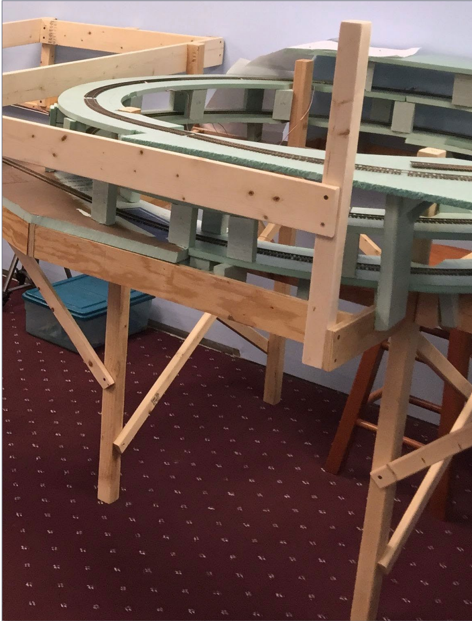
7. Helix wood benchwork frame with foam helix tier supports. The center remains open to permit access to the helix tracks.
