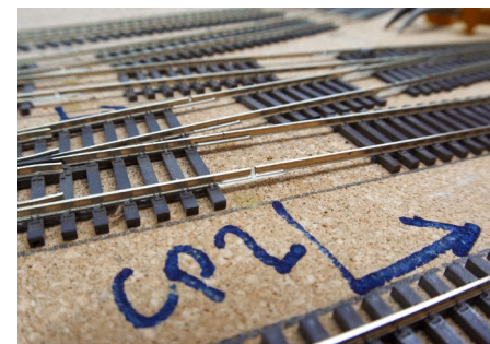
22, 23. The insulating rail joiners I used for the electrical gaps for detection. There is one gap in rail A (nearest to the fascia).
