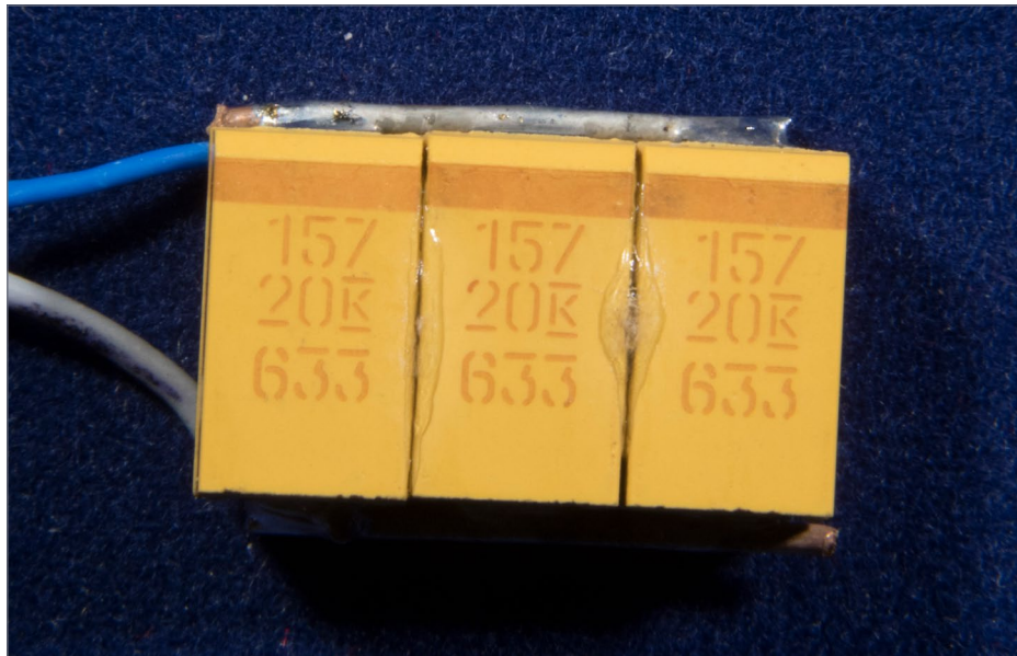
6. 450uF Ta capacitor "package." Three capacitors are glued together and wired in parallel, as seen from the top.
