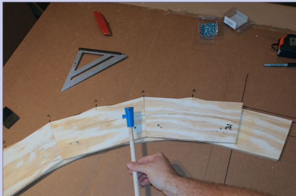
16. Before removing, I drew the track centerline on the top of each module tier.
