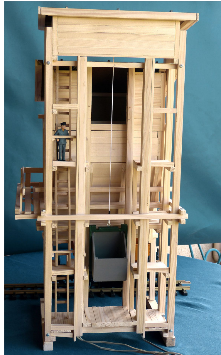
24. Hoist tower with bucket guides and hoist cable. The hidden wire channels are on each side of the hoist guide.
