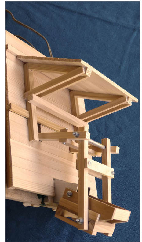
10, 11. Here is how the front face chute movement works, with the chute up or down.
