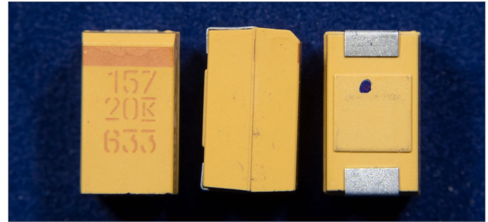
4. KEMET 150uF 20V Ta Capacitors, Showing top, side, and bottom. The solder pads wrap around from the bottom of the capacitor partway up the ends.
