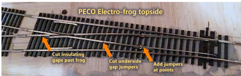
1. PECO Electro-frog turnout topside view with recommended wiring enhancements.
