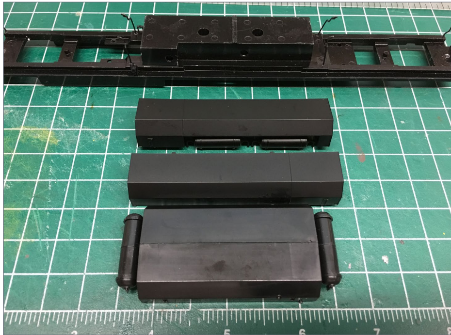
4. Comparison of the C40-8 and C30-7 fuel tanks next to the underside of the chassis. The C30-7 fuel tank will need to be "stretched" to the same length of the C40-8 tank.
