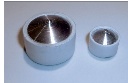
43. The masters for the mushroom-shaped roof vents, with turned aluminum centers inside plastic tube.
