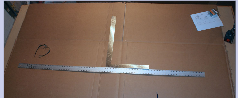
6. A large sheet of cardboard laid on a 4x8 sheet of MDF is the work area for a module template. A large steel rule and carpenter's square are used to establish the base and center lines of the module.
