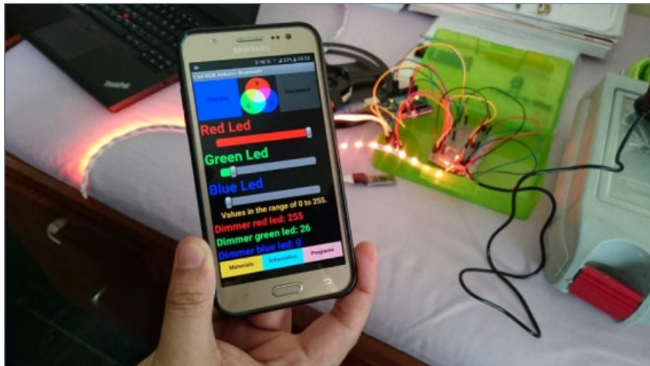
13. Arduino system test with digital control on the cell phone.
