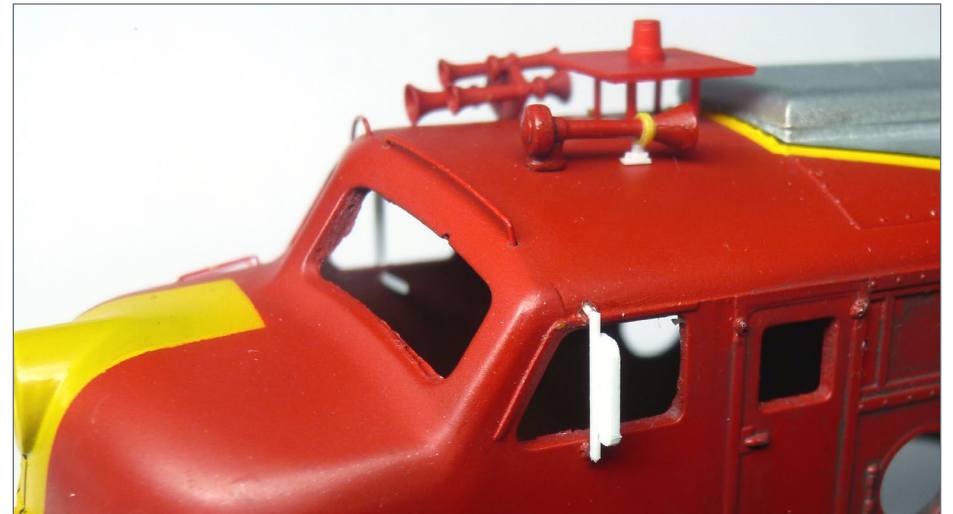
6. Air horns, grab irons, antenna with platform, and new mirrors were added to the shell between weathering stages.
