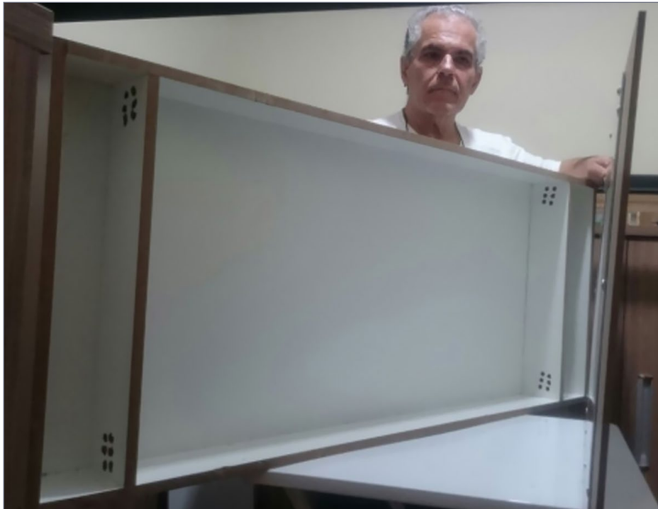
5. The basic backlight panel with a white interior.
