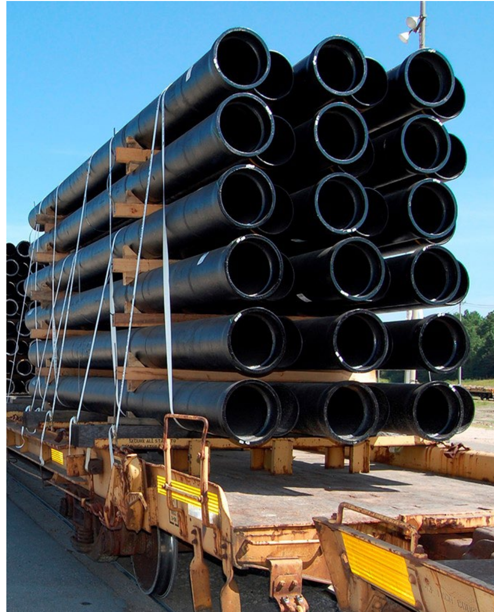
5. Another example of a ductile iron pipe load on a flatcar.
