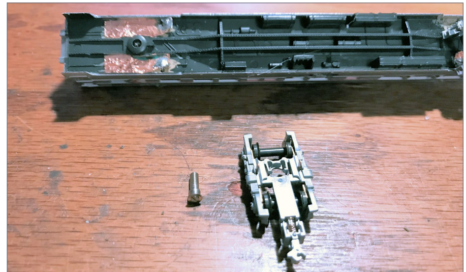
6. Copper foil applied to the smoothed-out area over the trucks.
