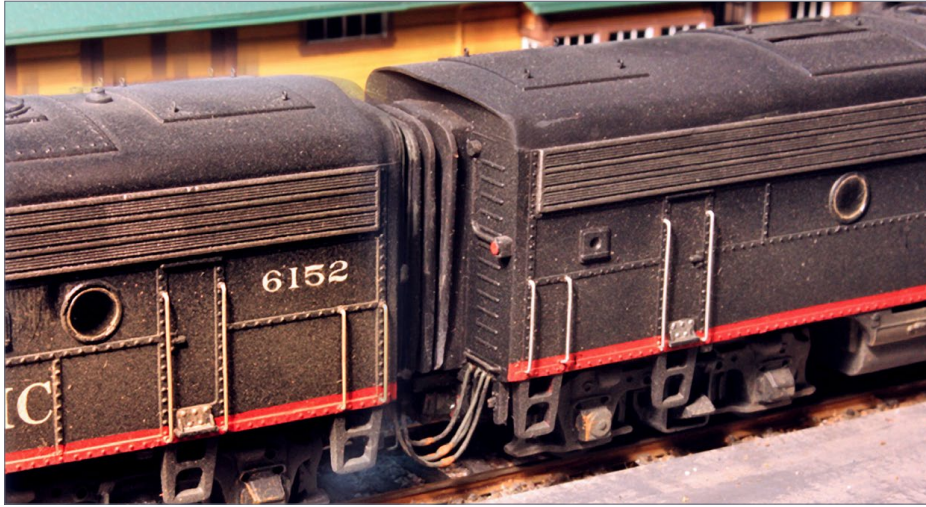
34. Here is how a pair of HO scale F units look with MU cable connections in place.
