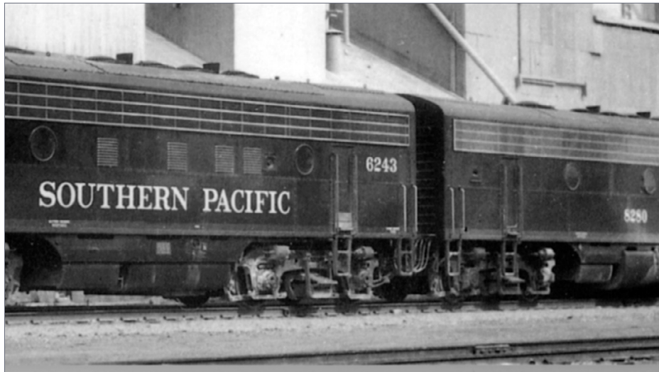
32. This pair of F7 units, shown entering Colton on February 18, 1956, have the usual multiple-unit (MU) jumper-cable connections between the A and B units. Detail of Robert E. Smith photo, Clark Bauer collection
