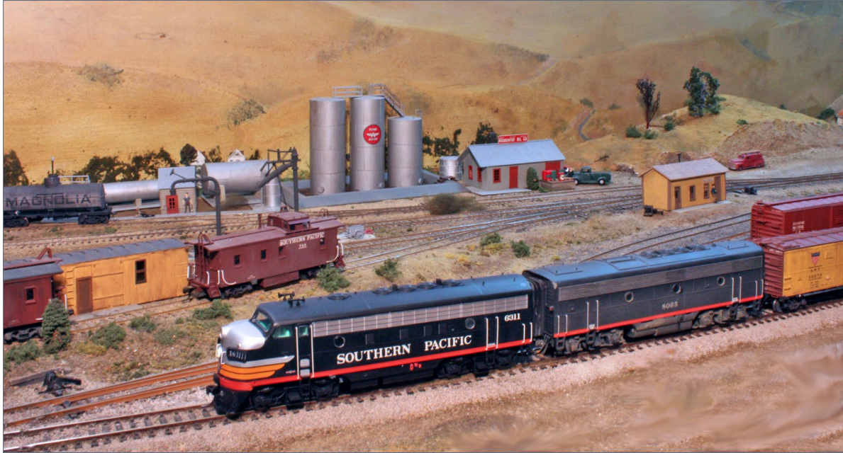
35. Models SP 6311 and 8065, shown passing Shumala on my layout, are both Athearn, but decades different in age; they are also, respectively, an F7-A and an F3-B. The units have a diaphragm between them, as was usually the case in 1953. The F3's dynamic brake exhaust slots are just visible, as are the MU cables between units.
