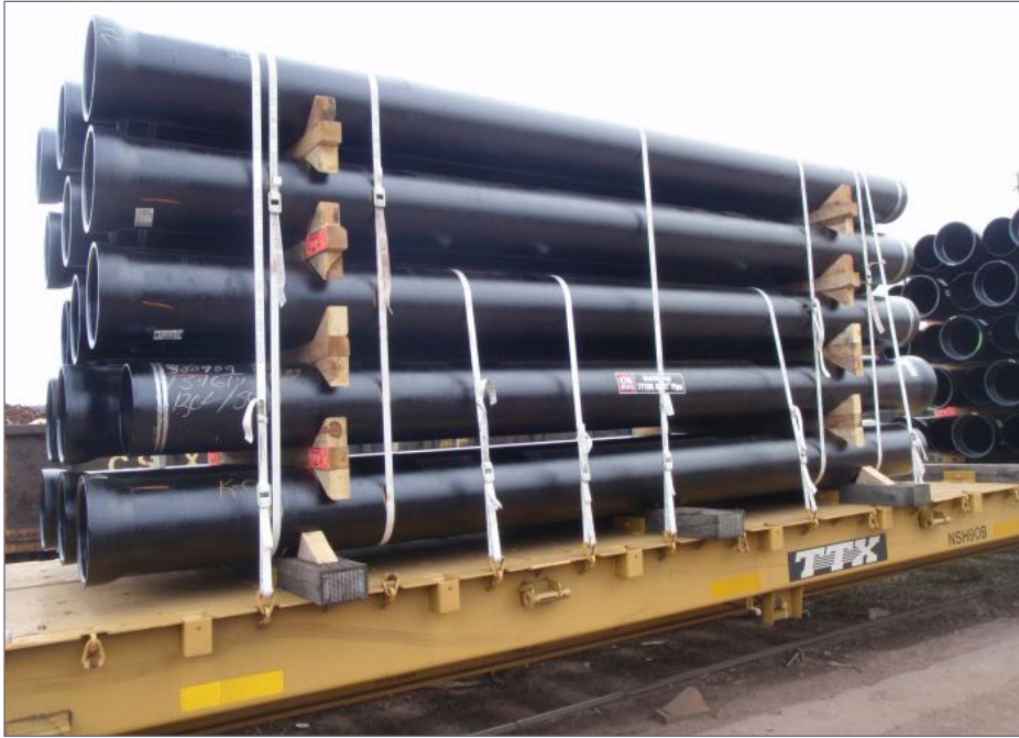
4. Example of a ductile iron pipe load on a flatcar.
