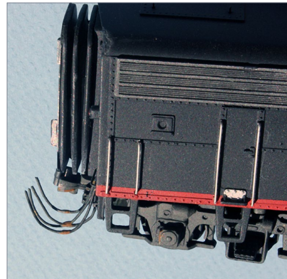
33. To represent MU cables, I use wires bent to an appropriate curved shape, with glue blobs at the bottom of the arc. They are attached only to the B unit.
