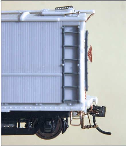
7. Close-up shows corner step with middle rung and other details including nut, bolt & washers added to ladder to match prototype photo.
