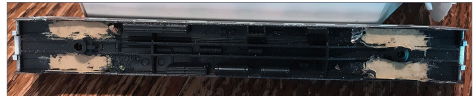
5. Altering the underside of the passenger cars to allow for Kato lighting contact tabs around the trucks.
