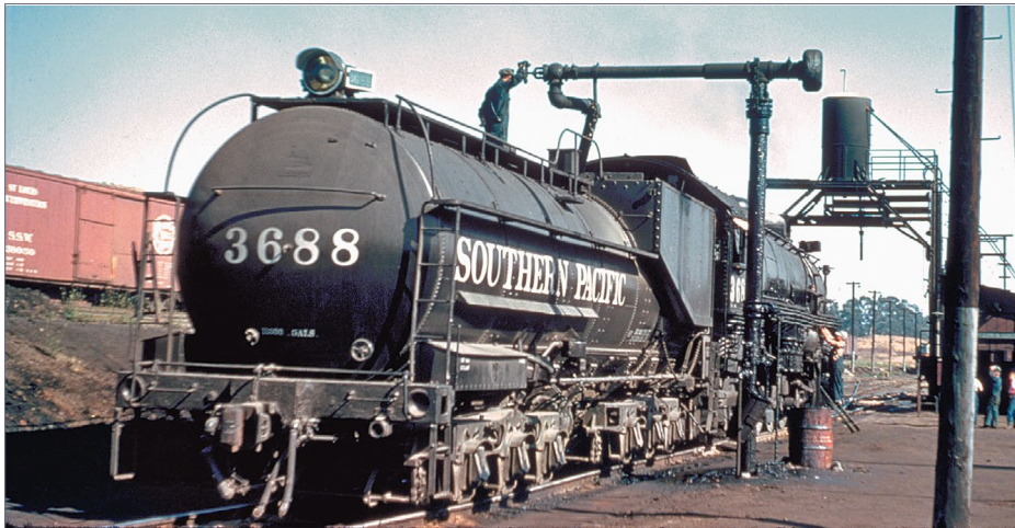
19. Among the many 2-10-2 helpers stationed at San Luis Obispo was Class F-4 3688. This image shows it being serviced after returning light from Santa Margarita. Here the tender oil bunker is being filled from a Rose oil column just south of the turntable; the overhead sand tower is just beyond the locomotive. The date is 1955. Alden Armstrong photo
