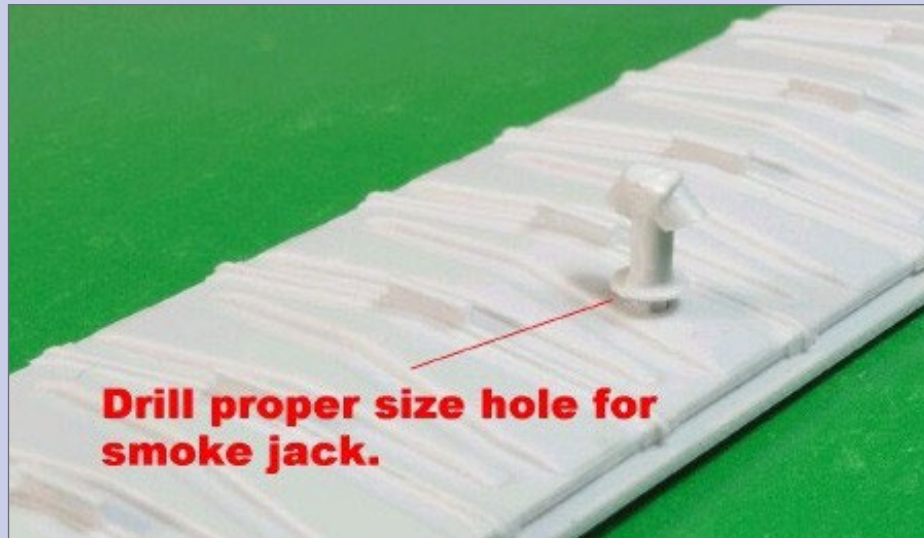
5a. Drill hole for smoke jack.
