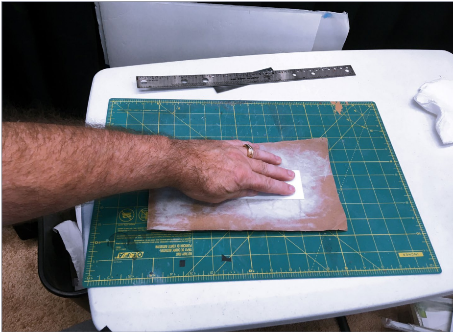
6. The door material needs to be sanded extra-thin to flex through the curving door track channel.
