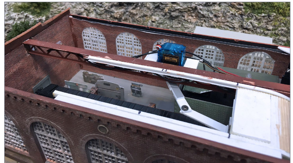
10. The servo, linkage, and door in the closed position.
