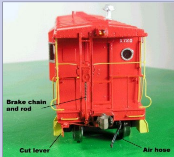
25b. Rebuilt end details.
