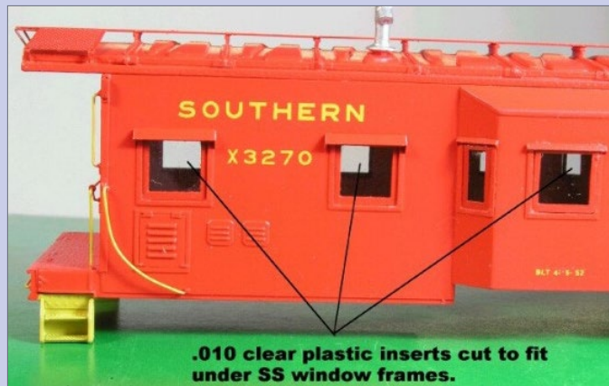
21. Clear windows installed from outside, counter to kit instructions.
