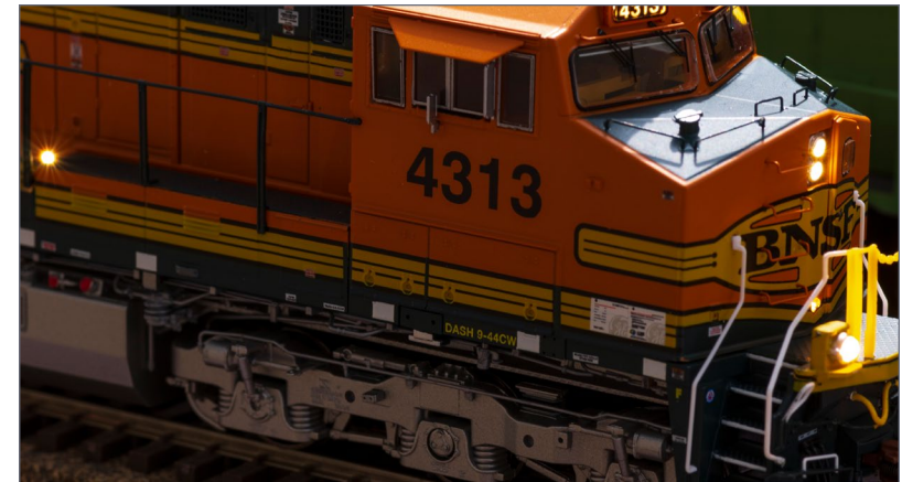
8. Illuminated number boards and front and side walkway lights.
