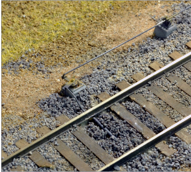
11. Looking more closely at the lever for the semaphore when the semaphore is in the STOP position. One of the carriers for the pipe can be seen to the right of the lever.
