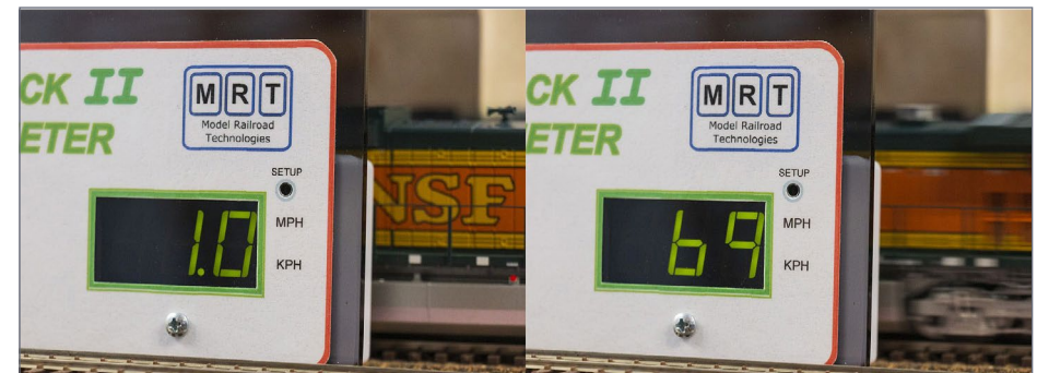
9. Speed trap results at slowest and fastest throttle settings.
