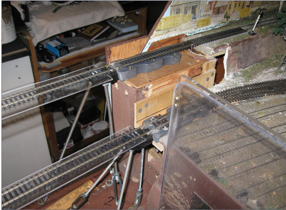
13. Socket block #2 in place on new threaded tripod screw framework. Socket block #3 below has a curved turnout on top. The turnout machine is 6" below the track.
