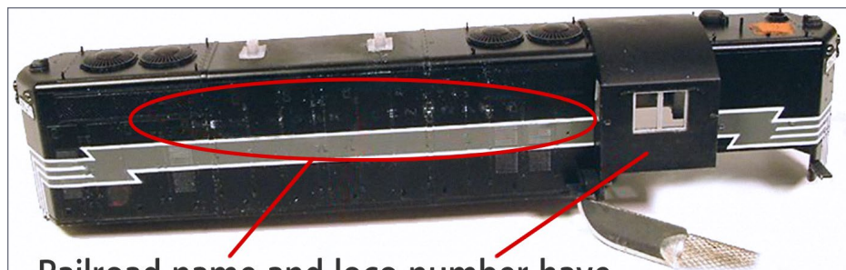
Railroad name and loco number have been removed by careful scraping and sanding
