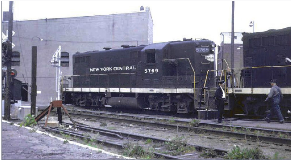
23. This color photo shows the bland cigar band paint scheme. This GP7 also has the 1600-gallon fuel tank.
