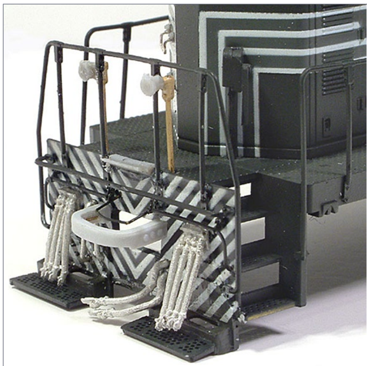
54. Here's the fully-detailed pilot, with MU stands, bumper, MU cables, and resin-cast footboards. Both ends are the same.
