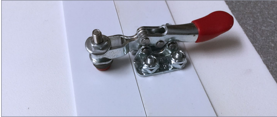
13. A close-up of the hold-down toggle clamp in the clamped position.
