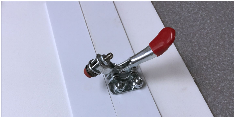
14. Here the hold-down toggle clamp is in the released position.
