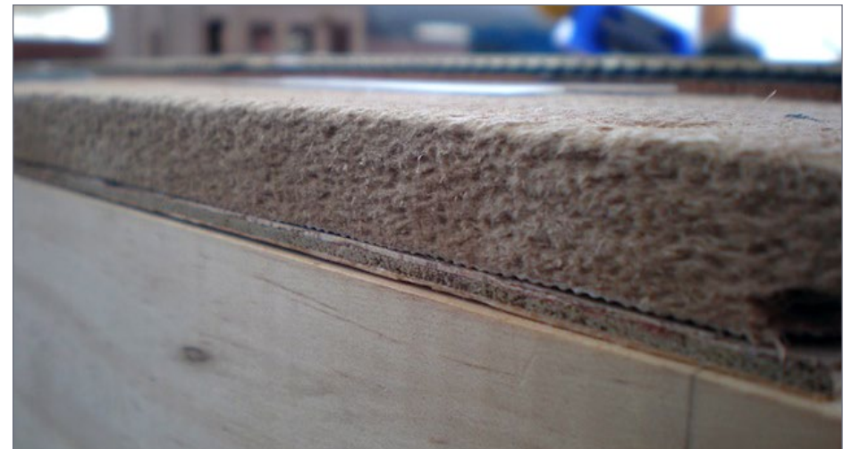
3. The lauan pine door skin and Canite sub-roadbed Jason used on his module.
