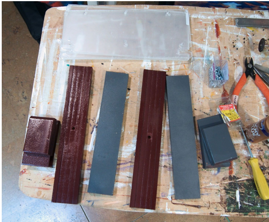
14. All the pieces for two cases, a top, bottom and two end doors and acrylic sides plus various screws.
