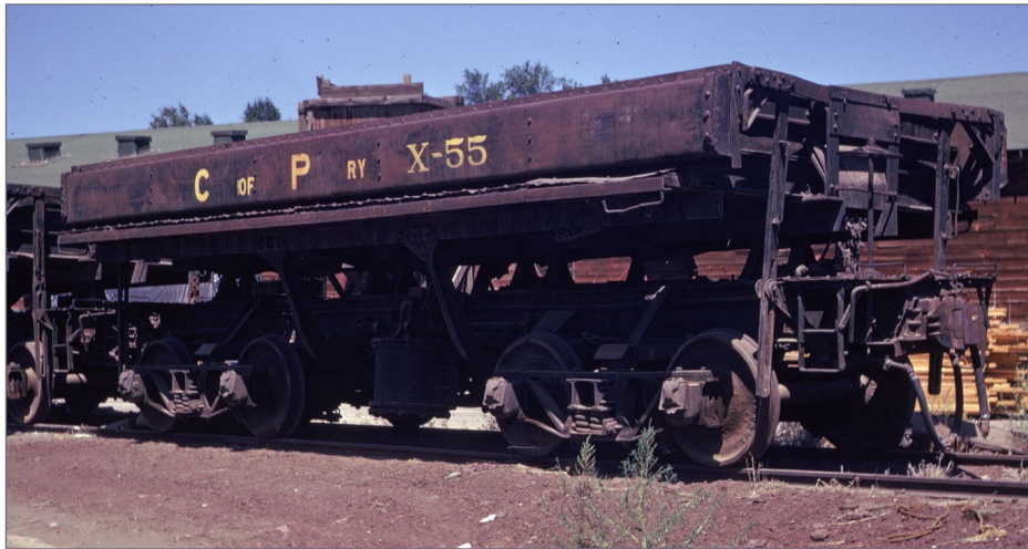
15. Here we see one of the two 20-yard Westin side-dump cars owned by the railroad sitting near the depot in Prineville in 1973. Photo by W.L. Hammond, collection of Gregory Baker
