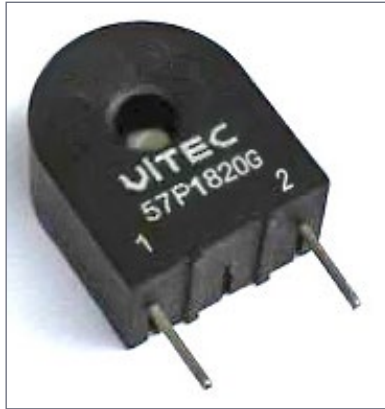
3. The Vitec 57P1820G transformer, which costs about $2.
