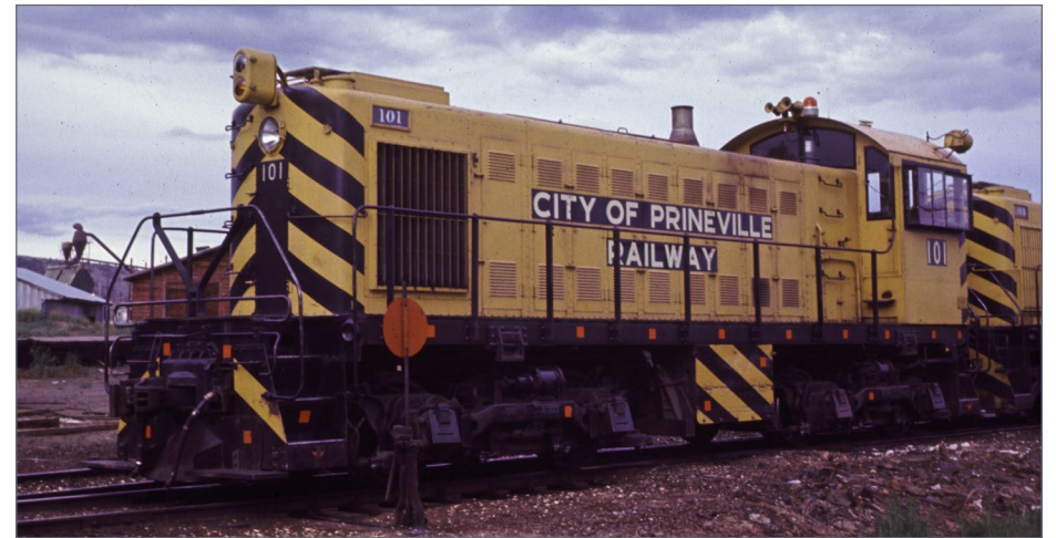
17. Alco 101, here in Prineville, was purchased new from Alco in 1950 and retired in 1984. The CofP added Gyalights and Mars lights to both ends of the units. These were activated when the horn was blown to provide additional visibility at road crossings. Photo by Gordon Lloyd, collection of Gregory Baker
