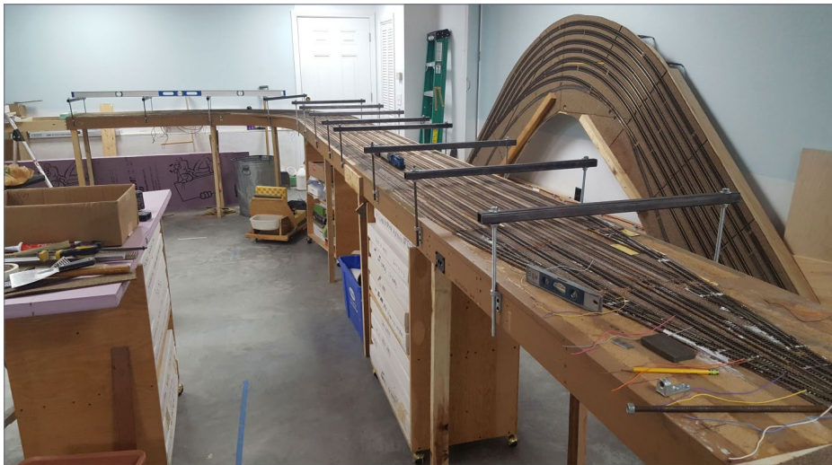
29. After the laborious task of drilling 3/8" holes in each end of the square tube at precise locations (using a drill press) – and the even more tedious job of threading all of the nuts and washers on the rods in the right sequence, I was ready for some help to restore the yard to its proper location.
