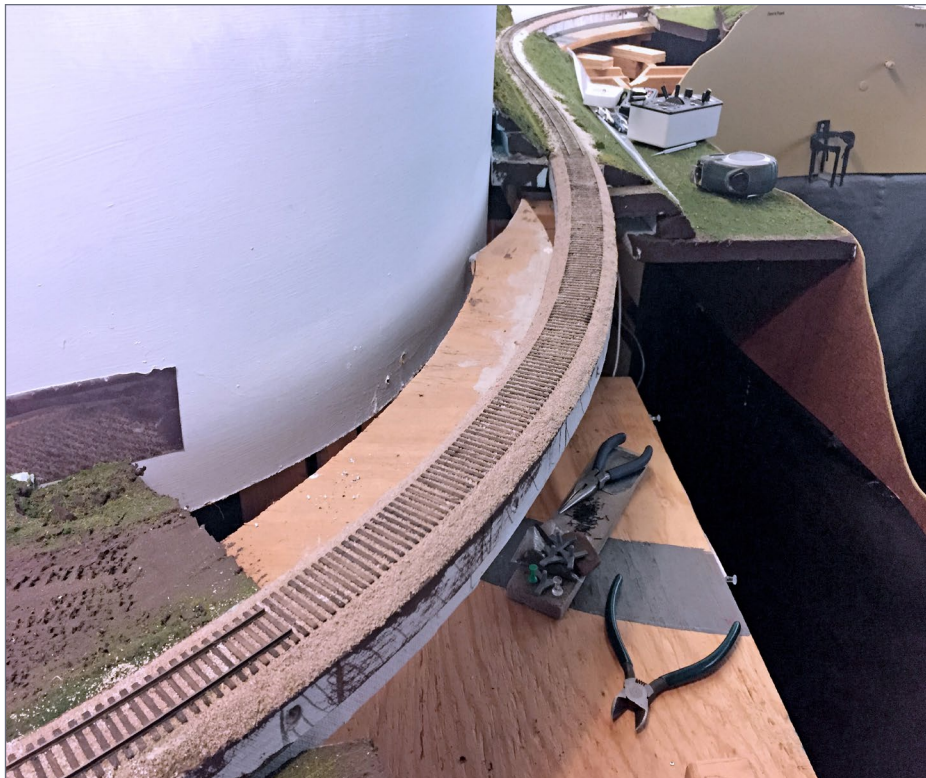
6. View of the High Bridge scene just prior to the removal of the Homasote splines. Rails have been cut, un-spiked, and removed.
