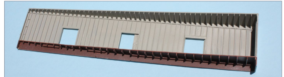
26. The "Light Sea Gray" color was spray-painted in the interior after masking all exterior surfaces, door edges, and the edge of the floor, to ensure the colors of those areas remained as originally painted.
