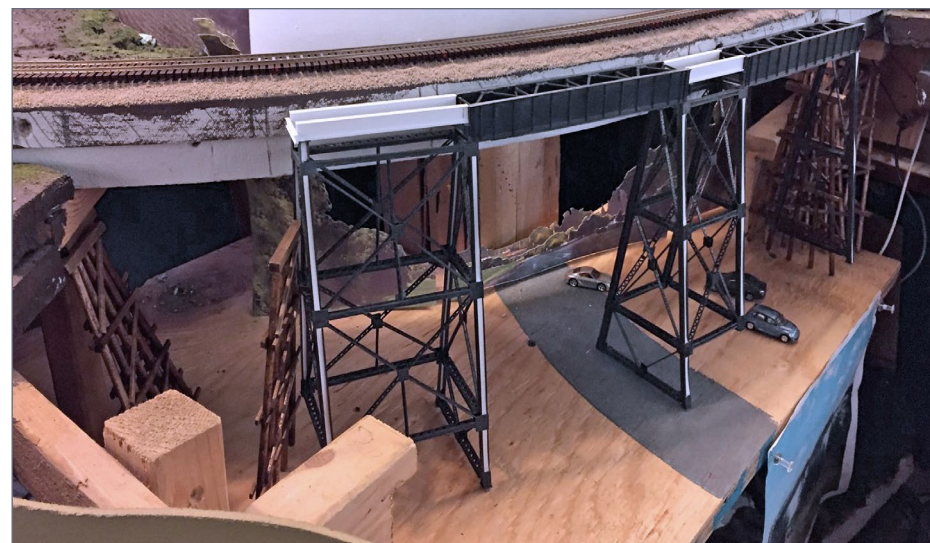
4. Micro Engineering bridge flex track resting on top of original spline and rail in order to form a template curve, with steel components of the bridge temporarily tacked together in the foreground.
