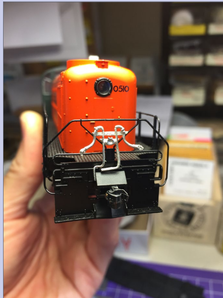
6. Cast metal MU stand securely held in place with contact cement.
