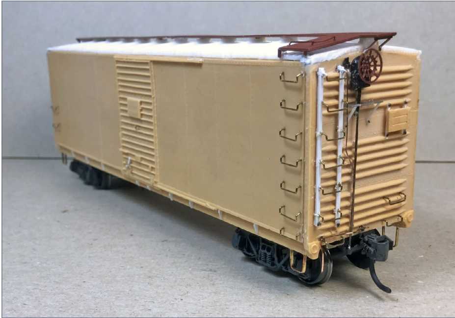
19. This resin boxcar model has a grab iron ladder on the car side and a grab iron ladder with stiles on the end.
