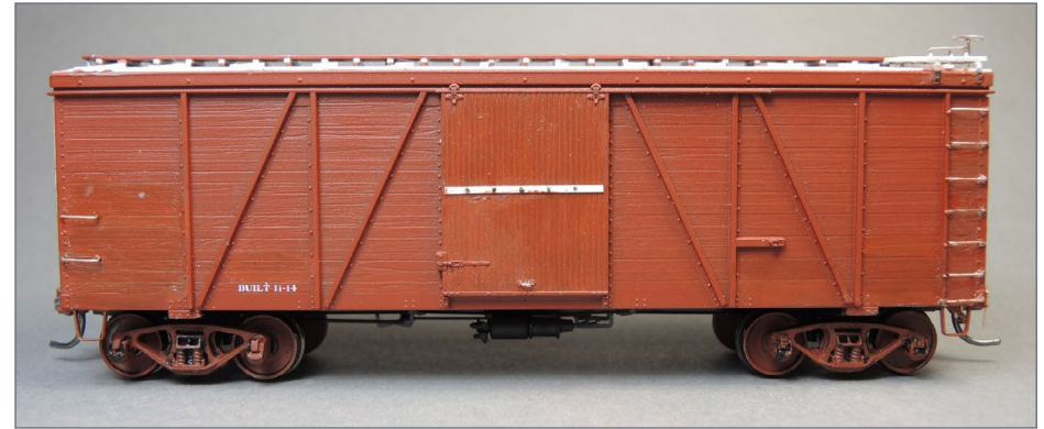
5. Several custom-bent grab irons have been installed on the right side of this boxcar.
