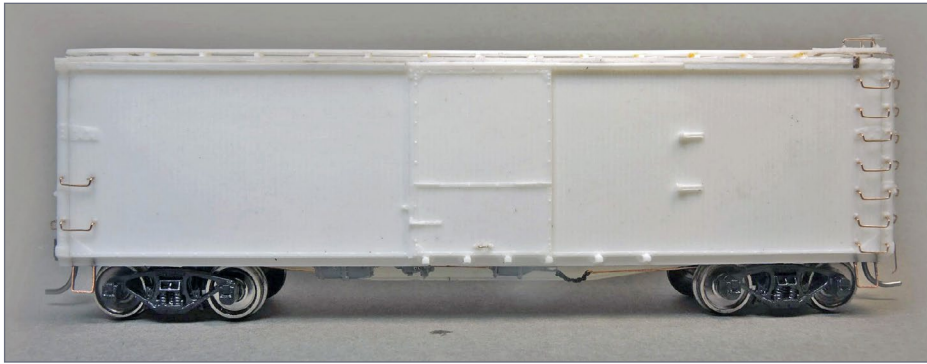
18. This resin boxcar kit has drop grab irons installed as the ladder detail.
