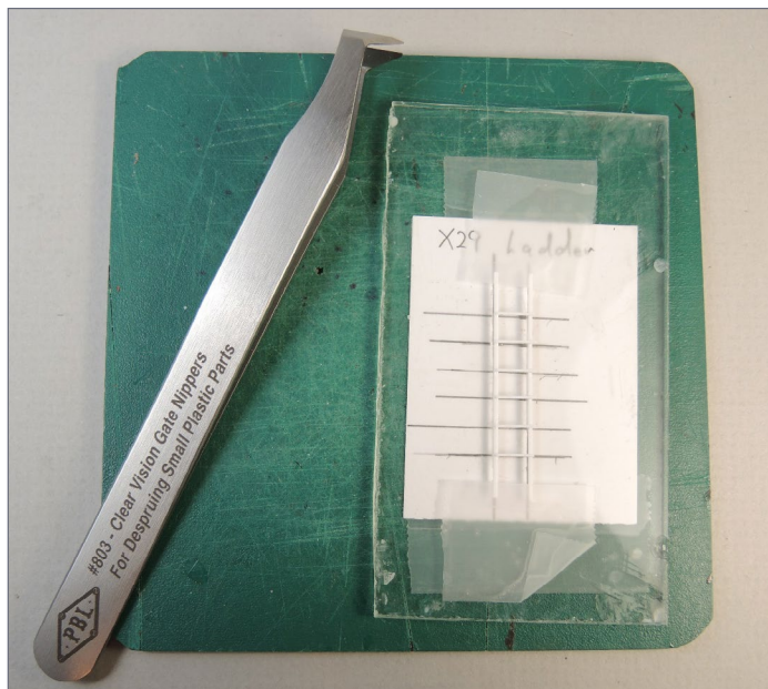
12. Use this sprue nipper to cut rungs to length. (Hold at 45 degree angle.)
