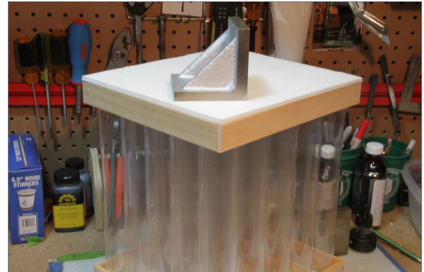
15. A piece of 8 \frac{3}{4} " x 9 \frac{3}{4} " foam board makes up the back of the organizer, preventing the stripwood from spilling out.
