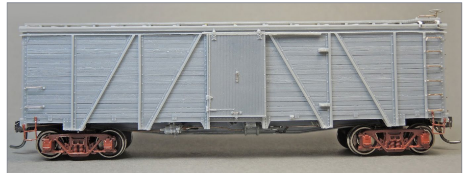
6. Ladder stiles are part of the car side casting on this Soo Line boxcar. Custom rungs are easily added.
