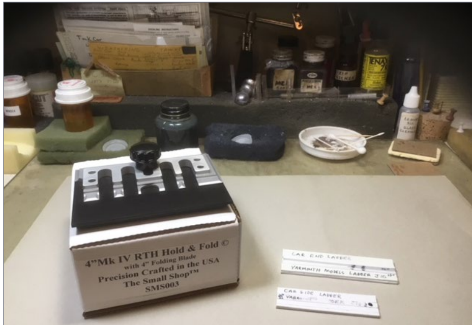
15. A Small Shop bending tool and the jigs I made for ladder assembly.
