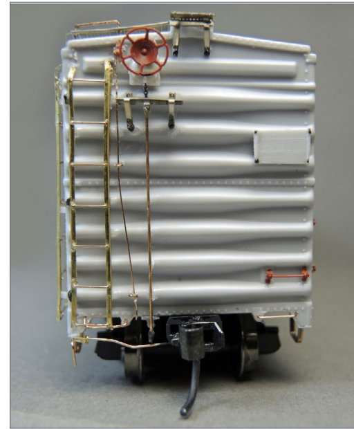
16. Brass photo-etched ladders installed on the B end of a resin boxcar kit.
