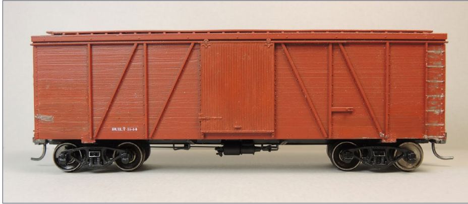
3. A plastic boxcar model with the molded-on grab irons removed.
