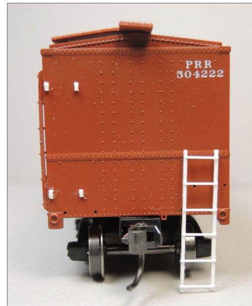
13. Here's a ladder is ready to install. Note the white ladder mounts on the car end.
