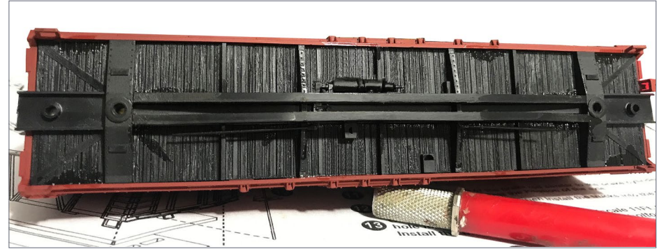
9. The floor is installed in the body and brake cylinder and brake rods with cranks are fitted and cemented in place. The brake rigging is from the Accurail gondola kit. These parts are available separately from Accurail in their parts listing on their web page.
