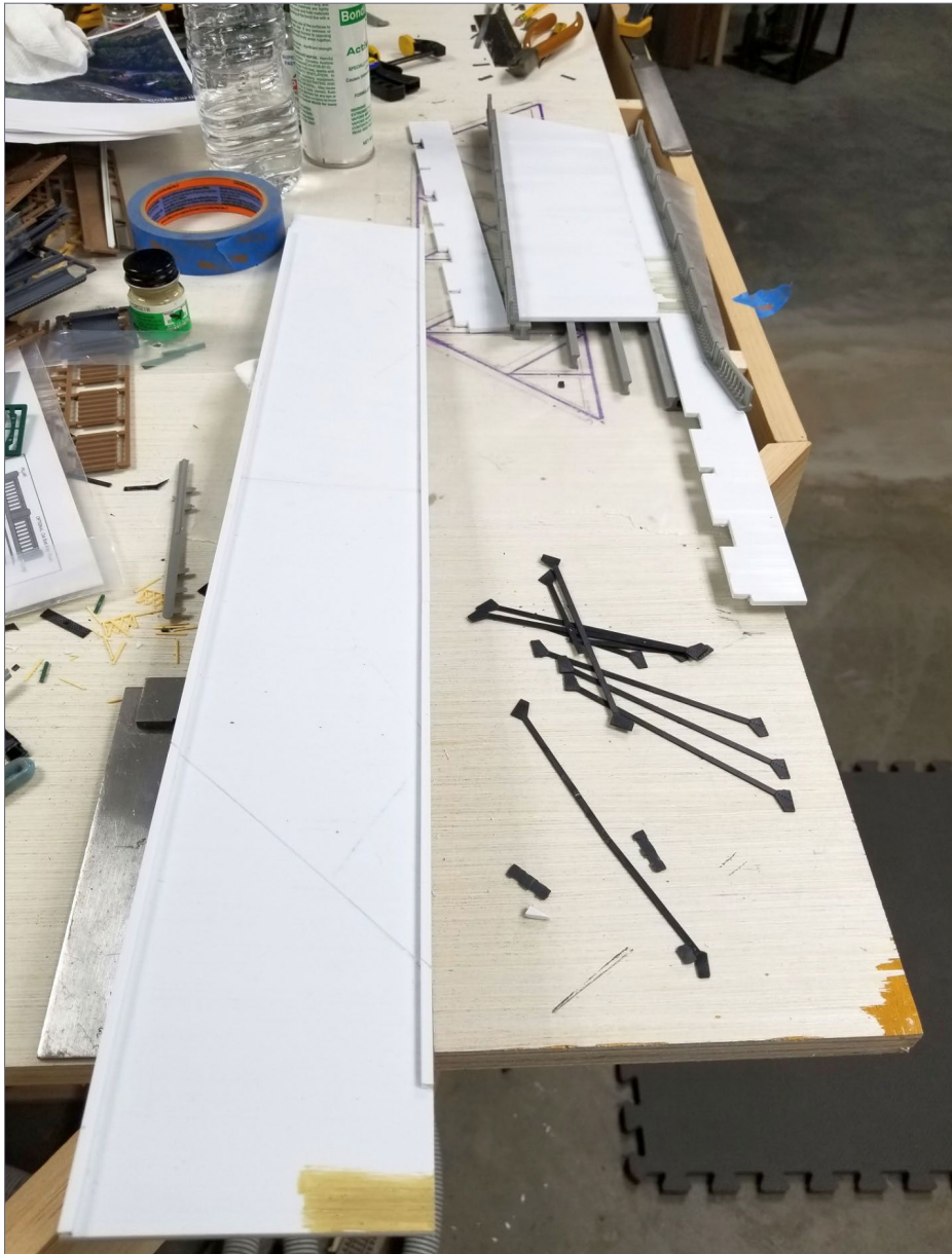
18. Here are all four pieces of the bridge deck/sidewalk system. Note the notches.
