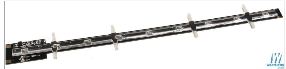
38. The Walther's DCC interior lighting kit fits into slots in the carbody.
