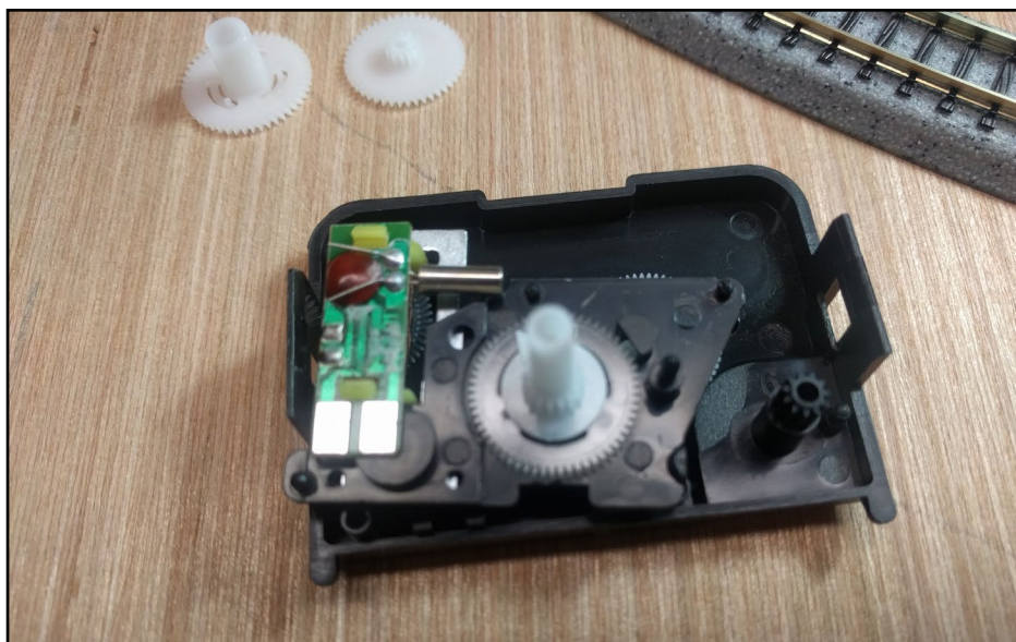
10. Further quartz mechanism disassembly.
