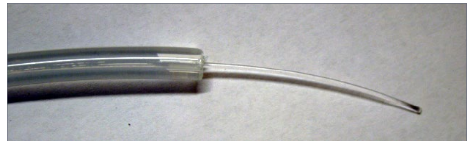
6. On the other end of the fiber optic cable, I removed about four inches of the nylon braiding. Then I carefully cut away several inches of the clear plastic cable casing to expose the bare fiber in the center.
