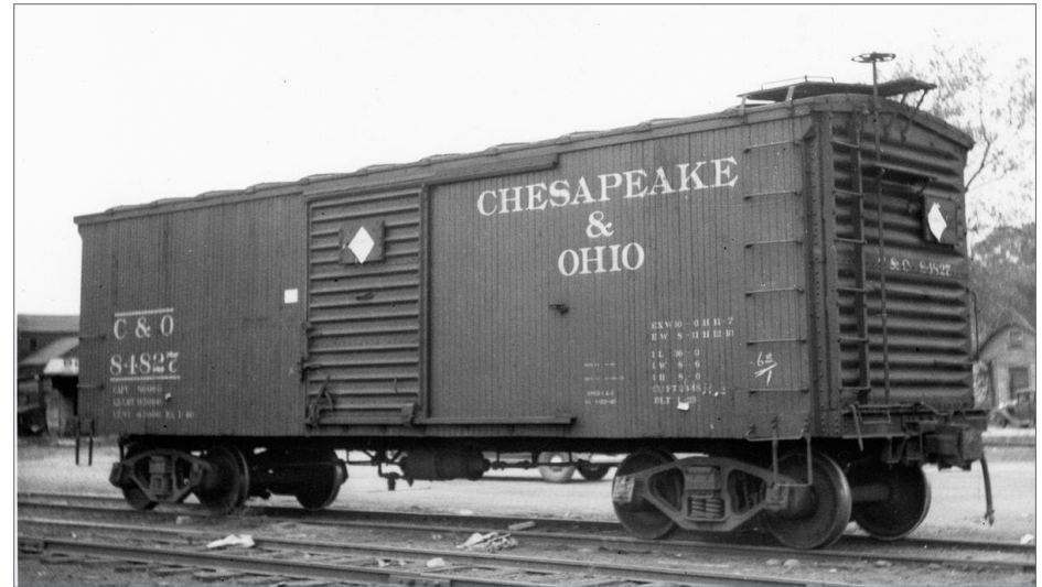
12. C&O cars rebuilt with Youngstown steel doors and radial roofs. C&OHS Collection
