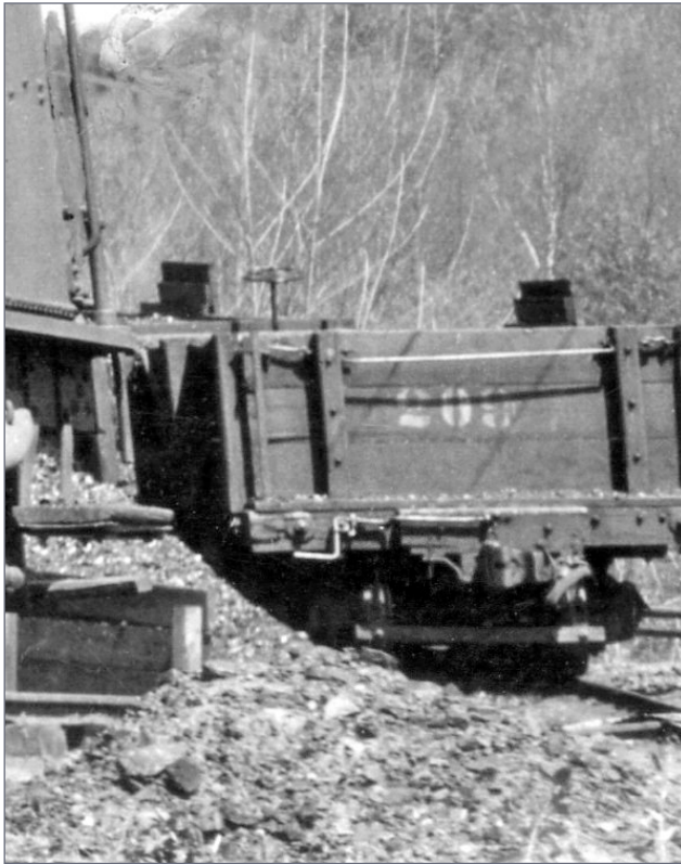
11. Gondola 209 in service. These gondolas may have been converted from flat cars.
