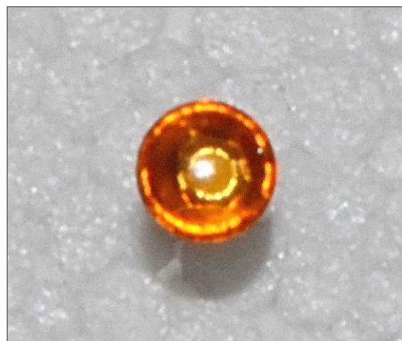
6. Closeup of the modified MV Products lens fits the A unit headlight housings.
