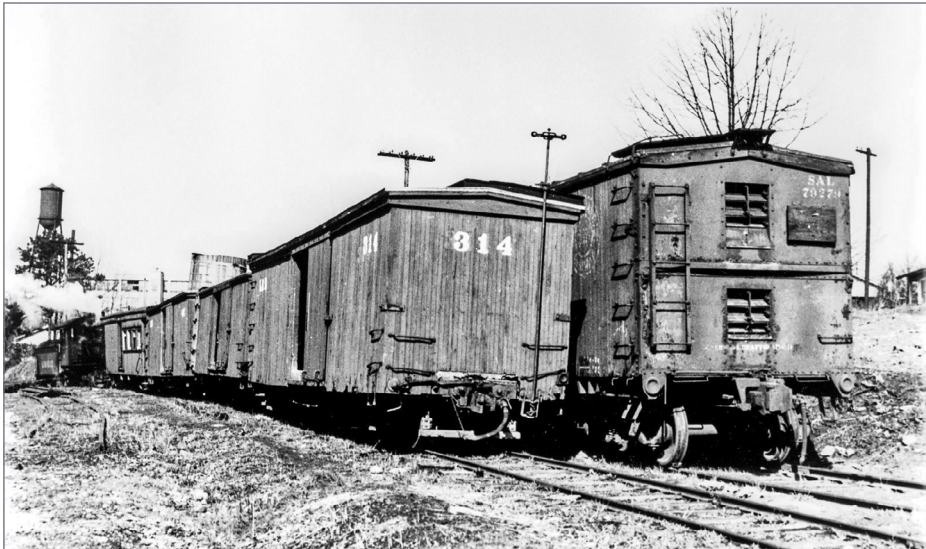
19. The interchange with the Seaboard at Lawndale Junction illustrates the size difference between narrow and standard gauge rolling stock. Collection of Donald R. Hensley, Jr.
