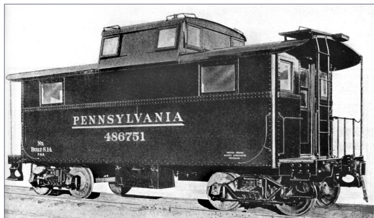
23. A builder's photo of PRR 486751, an N5 built in August 1914. Note the arch bar trucks and lack of collision posts. This is the first lettering scheme applied to both N5 and N6 cabooses. PRR Photo from the 1919 Car Builders Dictionary
