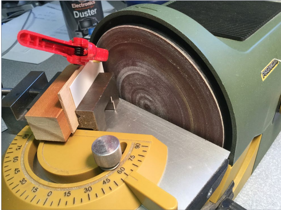
10. Grinding a piece of V-groove styrene to fit between an end window of the bay window 3D print and the front wall of the station.
