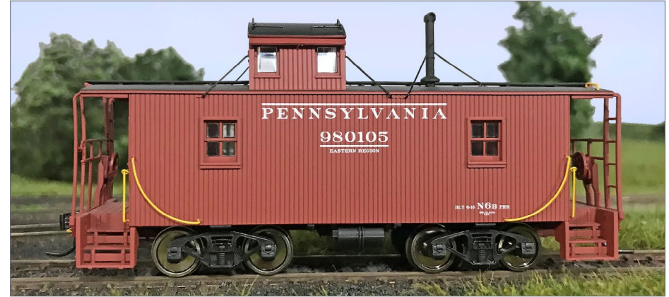
15. Here is the original Walthers Pennsylvania N6b caboose. It has the offset cupola, like most of the prototypes. Note the added guy-rod supports for the cupola and smoke jack. Compare this with the prototype photos [9, 10, 11].
