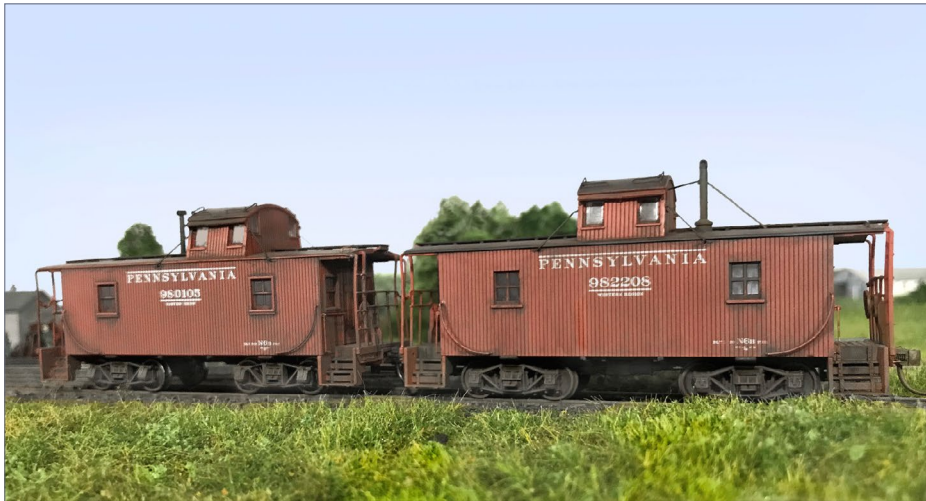
14. Here are the two Pennsy N6 cabin cars I prepared for this month's column. Both are Walthers models upgraded with Walthers arch bar caboose trucks, K brakes, and Kadee #153 couplers. The arch bar caboose trucks make a distinctive change in appearance for my 1920s scene.
