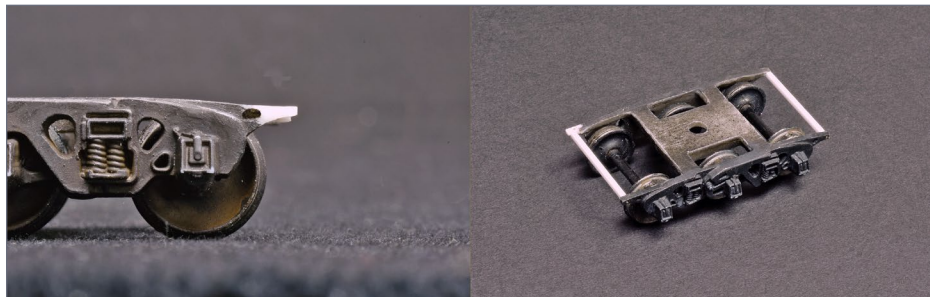
17. Repaired side frame and cross members fitted.
