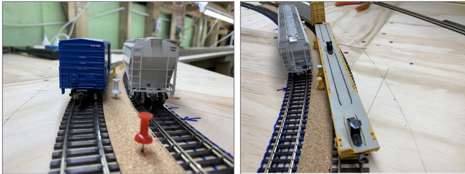
31a & b. Jason used the average length and maximum length rolling stock to check clearances.
