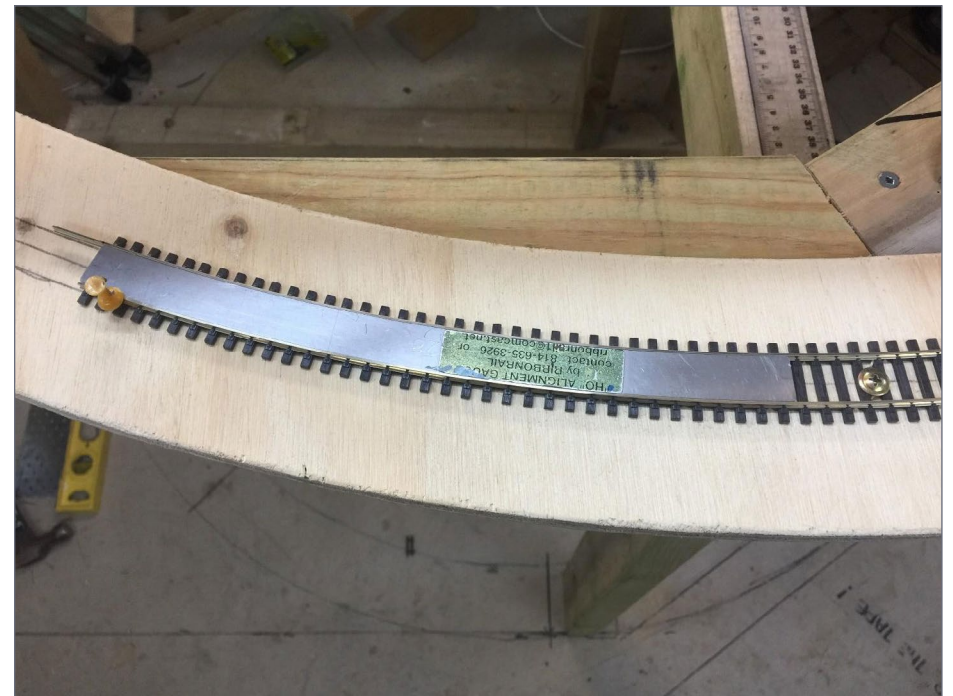
9. The RibbonRail Alignment Gauge used to set the 28" radius for the helix track.
