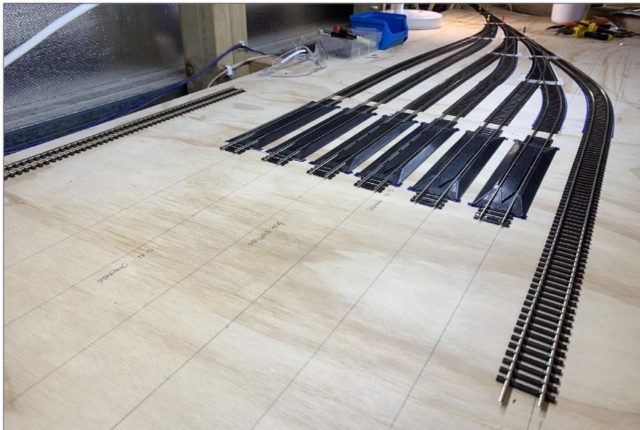
25. The staging yard ladder and rerailers connected together.
