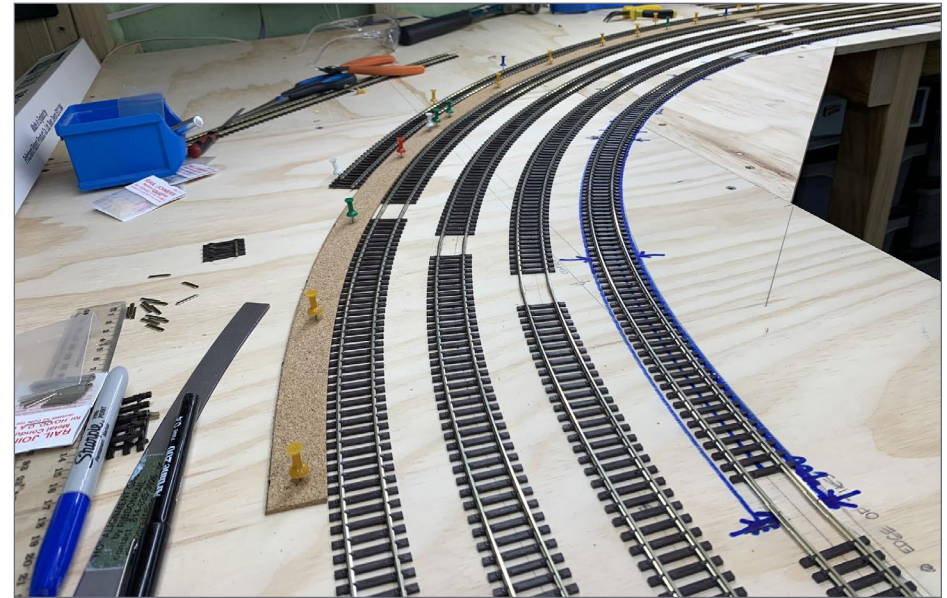
33. The cork spacer is simply secured using push pins into the plywood.
