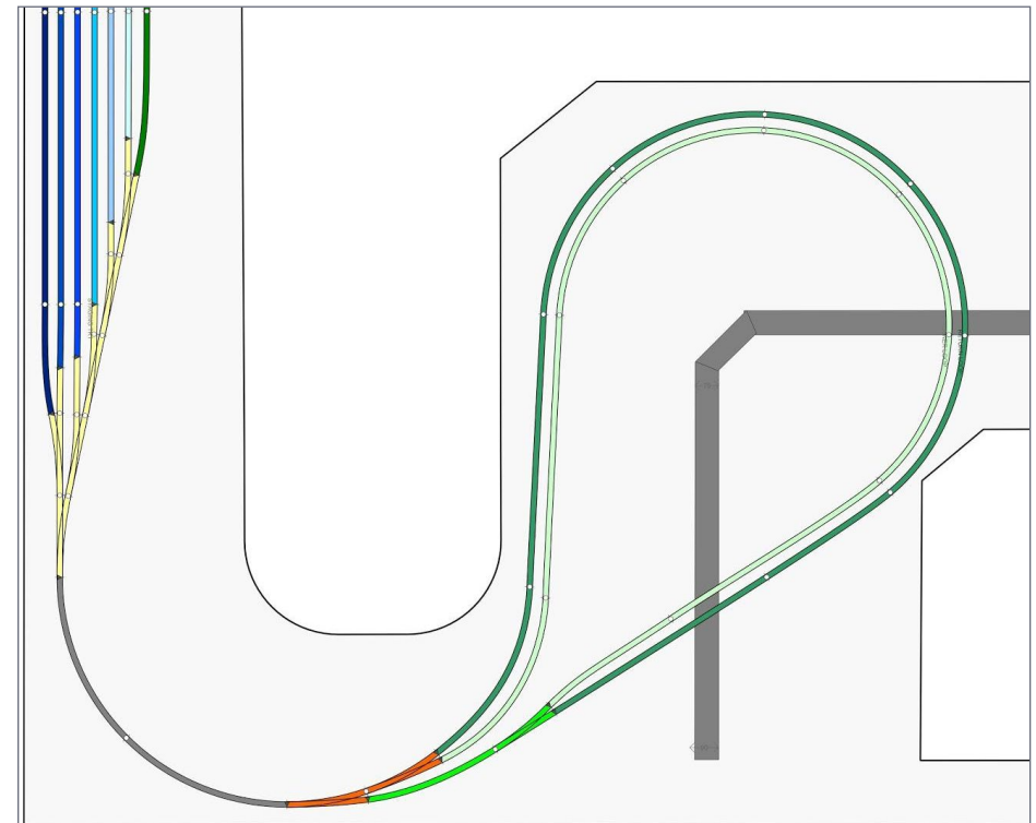
35. The southern yard ladder and 30" radius curve leading into the return loops.
