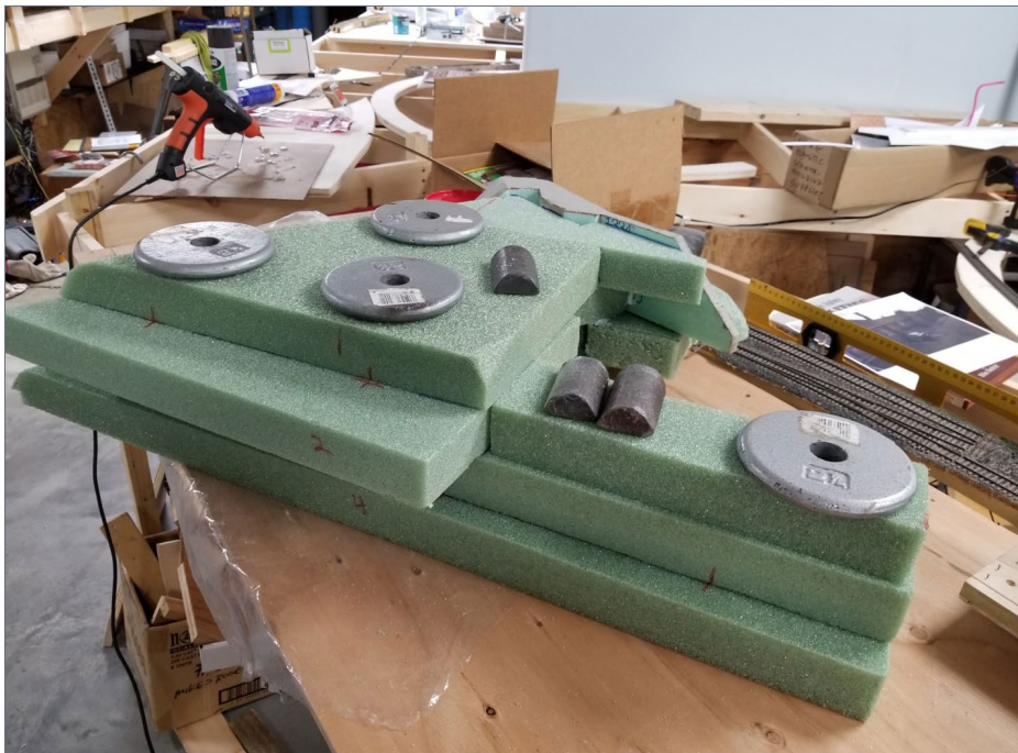
9. Weighting down the foam while the glue dries.
