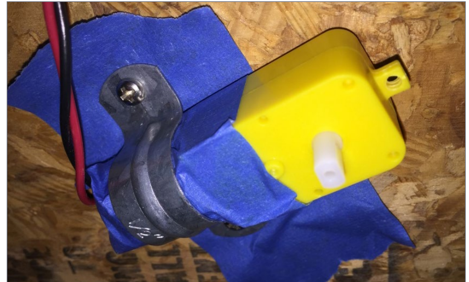
5. Attaching motor under the layout.
