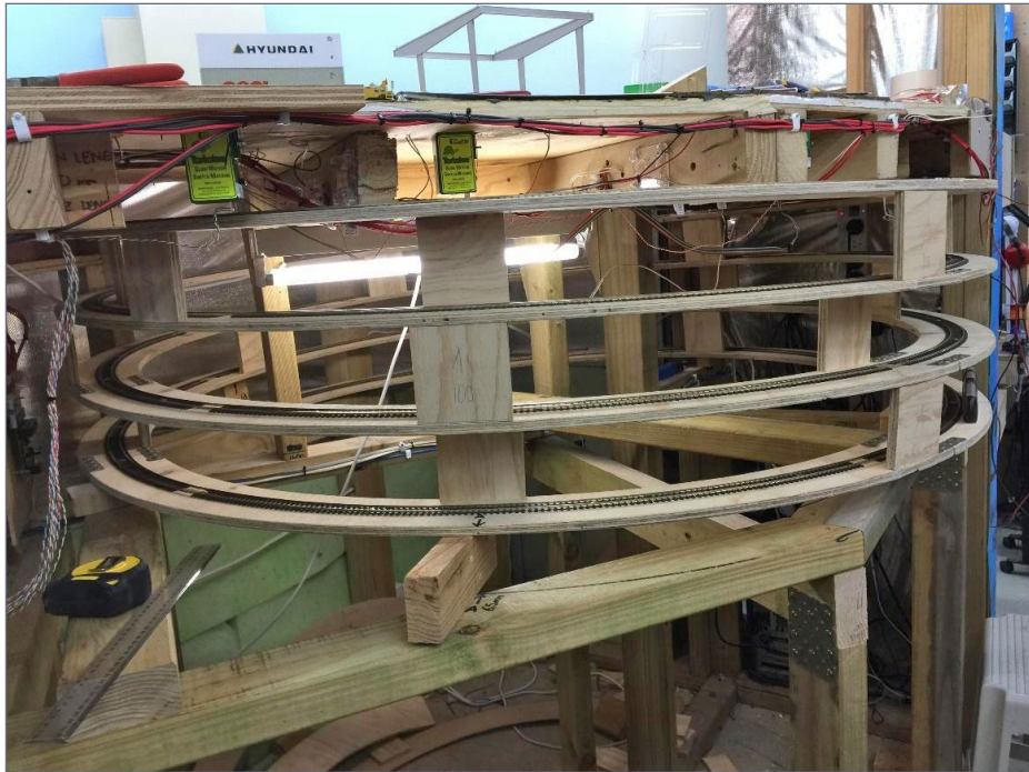
10. Setting the correct grade for the helix using spacers.
