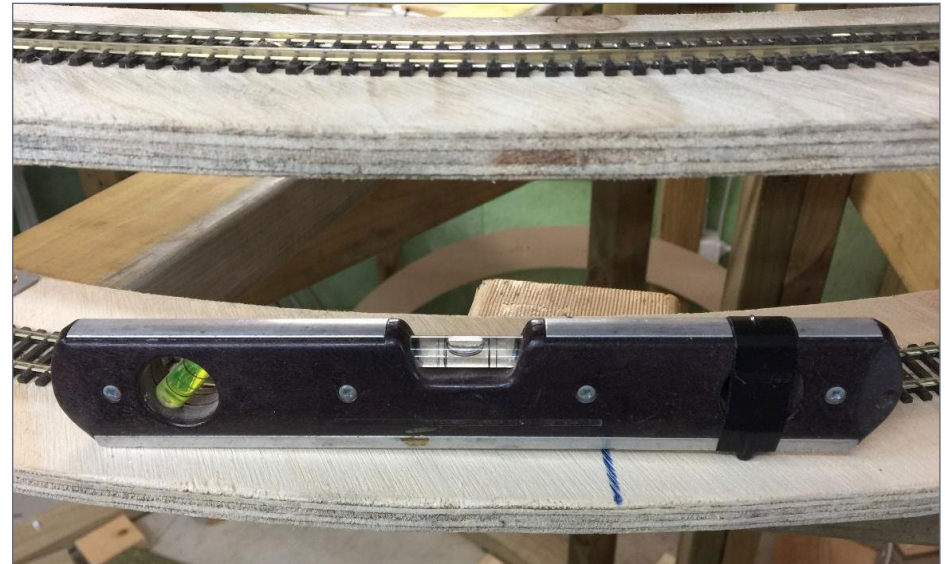
11. Jason's simple grade level he made for setting the first turns grade.
