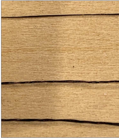
54. From top to bottom. EZ-Line fine, #38 magnet wire twisted, #36 magnet wire twisted.
