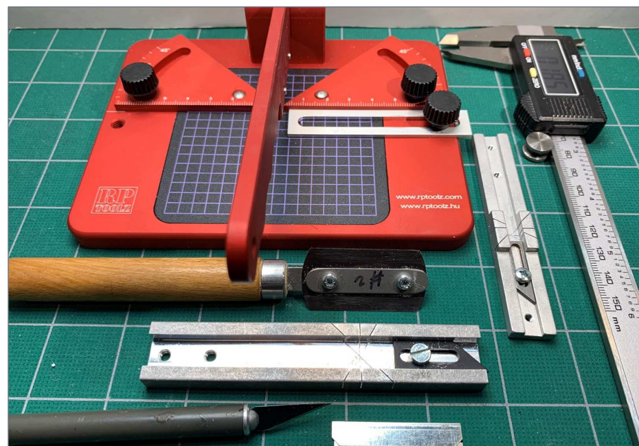
41. Sharp blades and accurate measuring tools are essential to produce the precise angles and dimensions for scale blocking.
