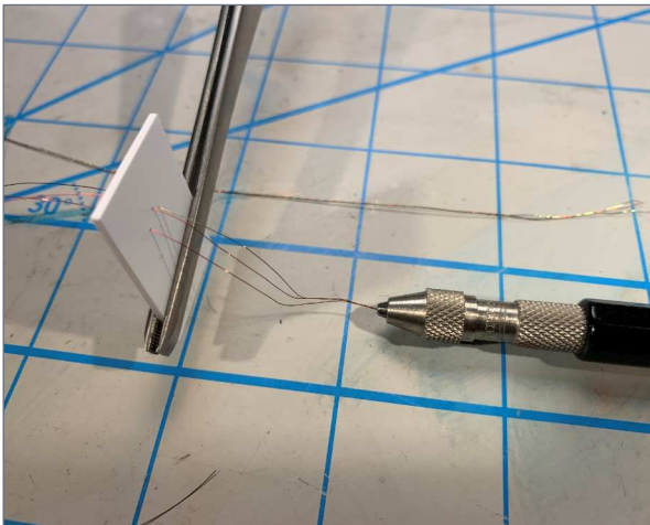
55. To simulate annealed wire, three strands of #38 magnet wire are threaded through the styrene guide and held in a pin vise.
