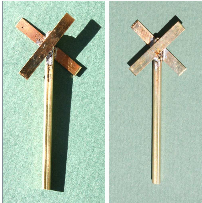
11. Two completed crossbucks, as soldered. Any excess solder will be cleaned up with a small file. The one at left does not have the post perfectly centered (note that the blade crossing is not exactly on the post), so I simply unsoldered and
