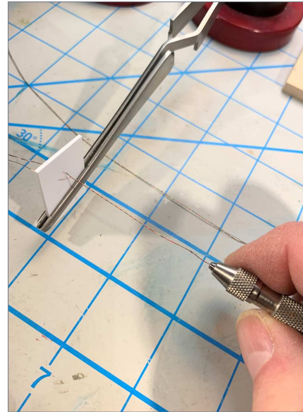
56. Putting the magnet wire under a little tension and twisting it forms the cable.
