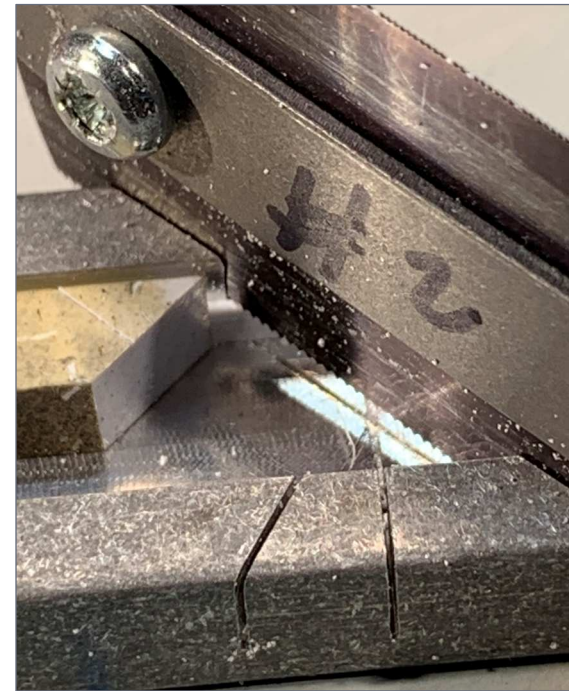
46. Cutting 2x6 styrene being securely held in the miter box.
