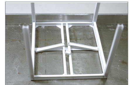
29. Cut and fit and glue single cross beam.
