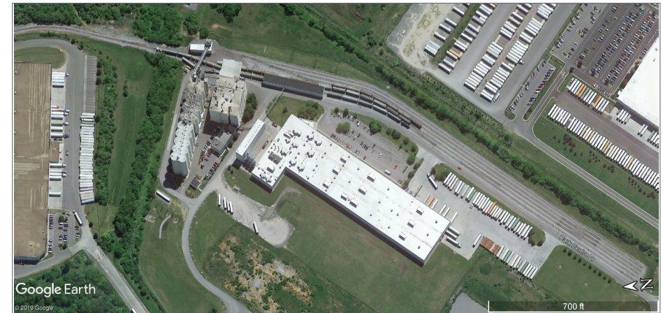
26. The Miller Milling grain mill is served by CSX unit trains on a nearly weekly basis. Look at the crossover switches at the south end of their storage tracks, allowing locomotives to escape to the next track. Google Maps
