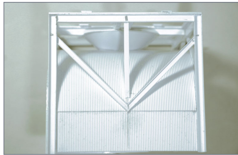
39. 1/8" H-column and 1/8" I-beam angle braces added to the scale house side of the base.
