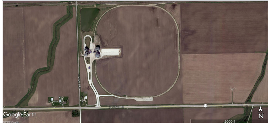
11. The Consolidated Grain and Barge Co. grain elevator facility with loop track near Dwight, Illinois. Notice the placement of the metal bins: some inside, some outside the loop track. Google Maps
