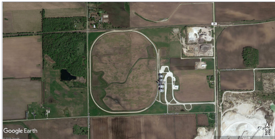
12. The FS Grain elevator facility with loop track. Here the grain bins are in a single line outside of the loop. This facility also has a small storage track branching off the loop. Google Maps
