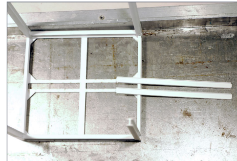
28. Cut and fit and glue double cross beams.
