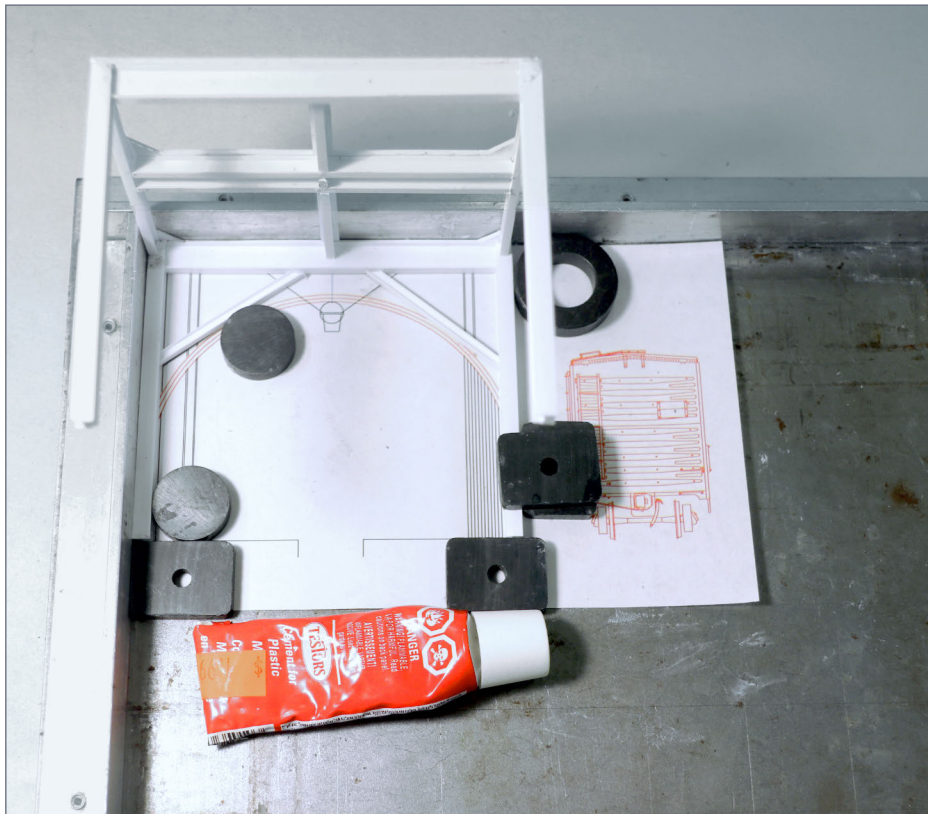
30. Fit angle I-beam braces to the ends.
