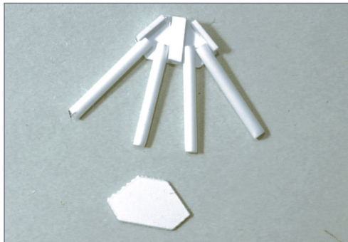
36. Assembling the distributing head. The tubes helped position and space the components but were not glued into the assembly.
