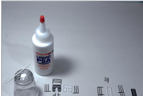
52. Walkways were assembled with PSA.
