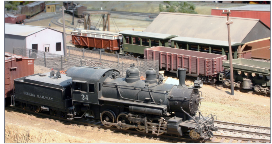
3. A brass NWSL 2-8-0 modified to represent the Sierra Railway number 24. Three scratchbuilt open excursion cars sit the on the siding in the background.
