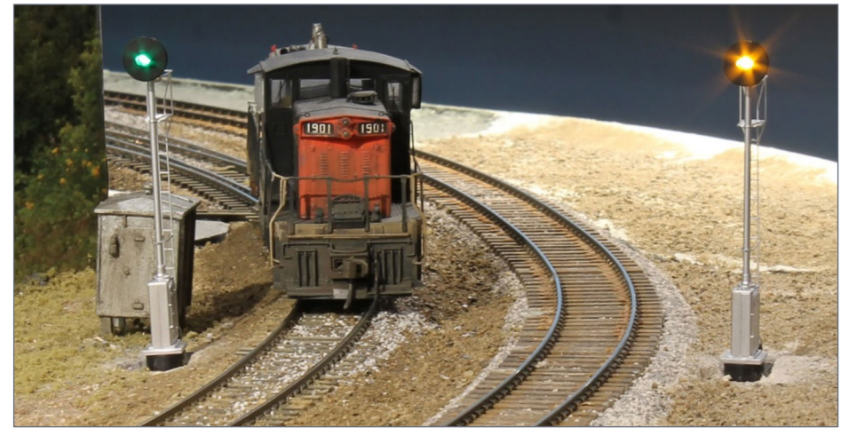
9. Two Signalman-S outputs drive two BLMA target signals. Each signal head has three individual LEDs.
