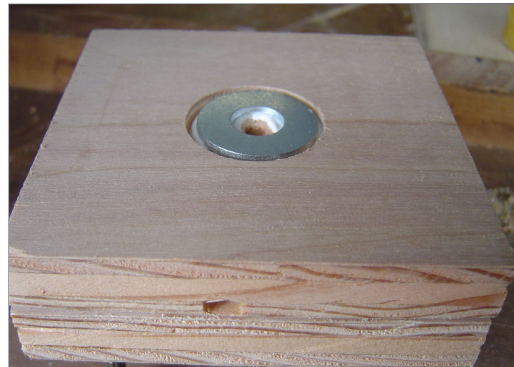
11. The final step was placing the washer into its shallow hole and securing with adhesive caulk.
