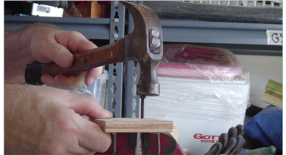
7. With the holes drilled through, it only took a few taps to put the nails in.
