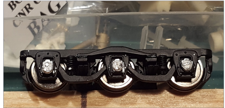
18. All finished, with roller bearing wheelsets. I questioned my sanity when I began upgrading such small parts, but I think it was worth it.
