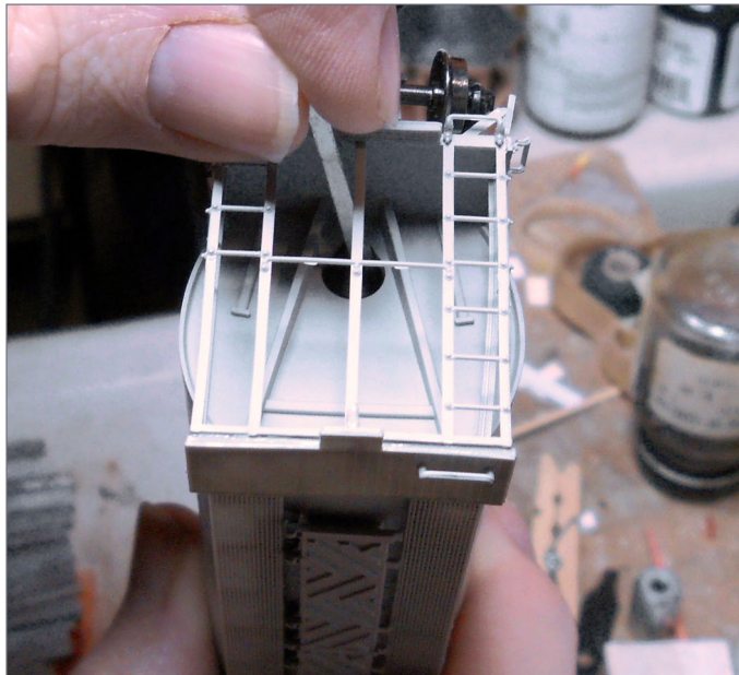
15. Weight bars through the hole.
