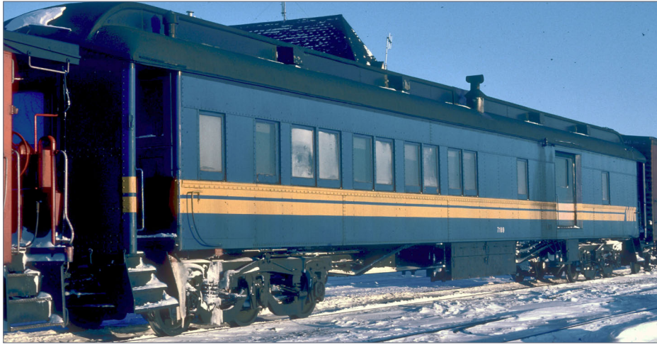
3. VIA Rail Colonist combine no. 7189 is stopped at the Churchill, MB, depot in January 1987. The view is of the battery-box side. Note that the coach's original trucks have been upgraded with roller bearing axles. Mark Perry photo
