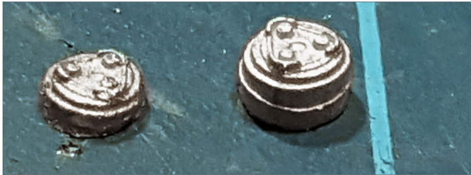
17. The original roller bearing casting is on the right, and my trimmed-down version on the left. This task became easier and quicker as I learned what I was doing. This was a good thing because there were 12 of them.
