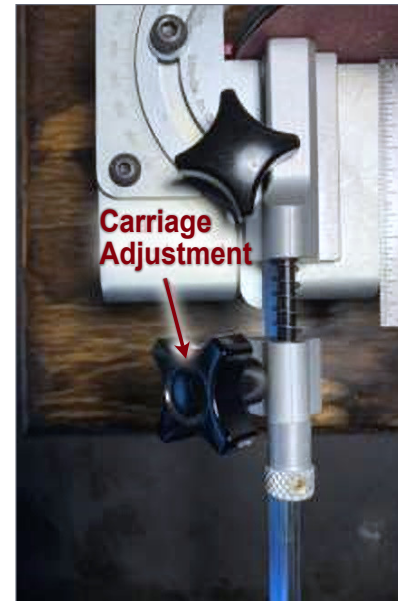
13. You must slide the carriage adjustment back all the way to verify quadrant alignment.
