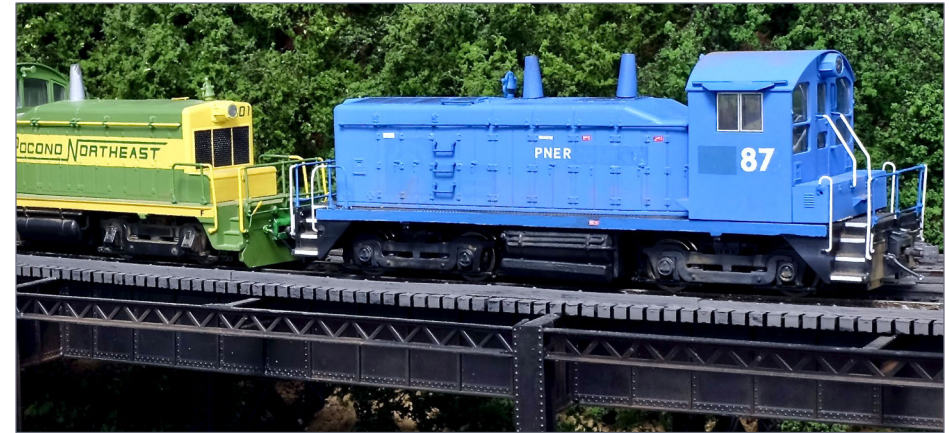
2. The finished PNER no. 87, modified with a Walther's Proto chassis and detailed to look like the prototype [1]. Note the SW1 in the attractive PNER paint scheme coupled to 87.
