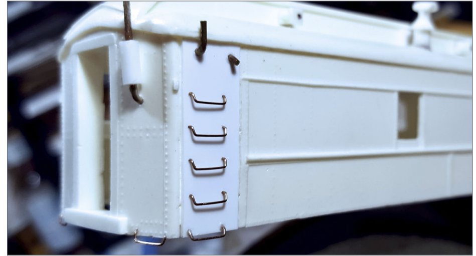
8. I plated-over a vestibule door and added fuel filler, fuel vent, and smokestack details to represent a generator that CN installed in the baggage end vestibule of the combine. Note the five-grab ladder. I used a template to achieve an even 18" scale spacing between them.
