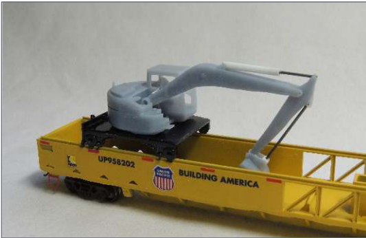
24. Test-fitting the excavator and crawler cart to the car. Note the styrene and wire hydraulic ram on the boom.
