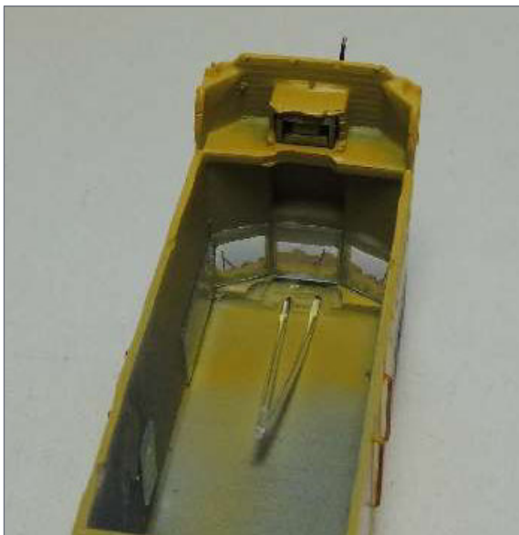
9. Windows and fiber optics are installed in the control cab. Ready for the interior.
