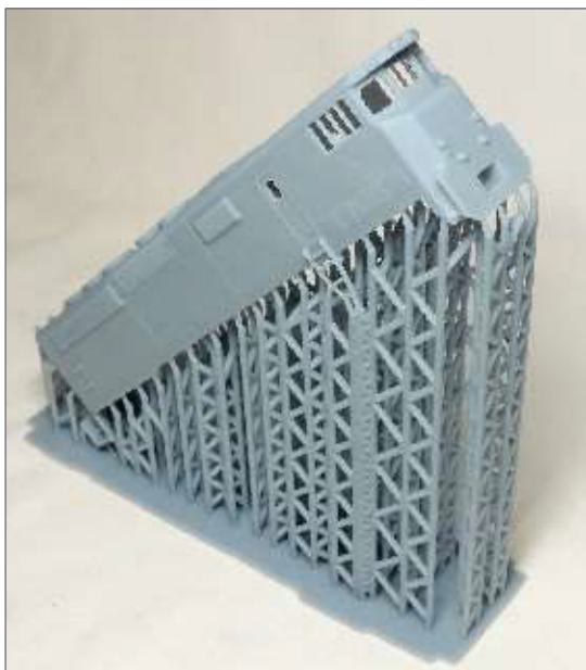
26. The rebuilt SD40-2 fresh off the printer.
