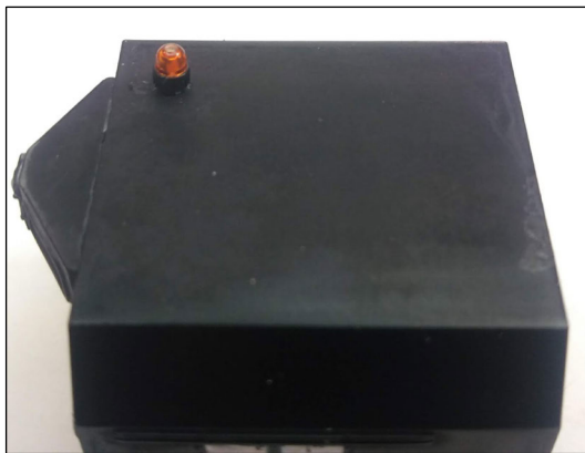
17. The LED is mounted to the cab roof of the locomotive, on the engineer's side.
