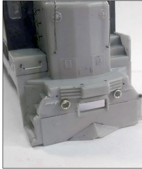
21. I used 3/32" brass tubing for the ditch light housings. Here they are shown secured with CA adhesive in the front pilot holes.
