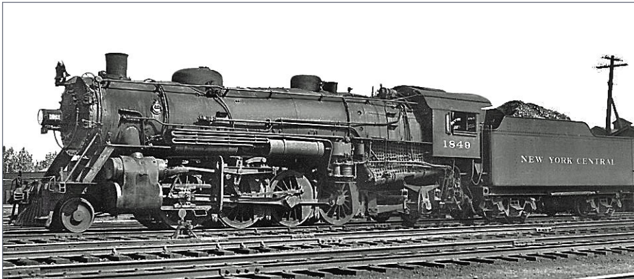
24. This view of NYC H6 1849 is typical of 1937 to about 1940 with the Roman lettering and the 1849 number. NYC locomotives were renumbered in 1936. Note the poling pole alongside the tender frame and the lack of cab roof wind deflectors. Ray Breyer collection
