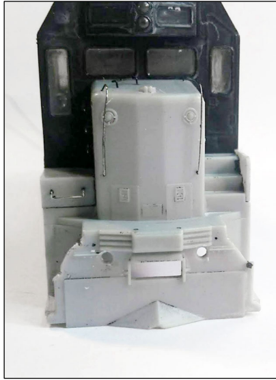
20. I drilled holes for the ditch lights in the pilots.
