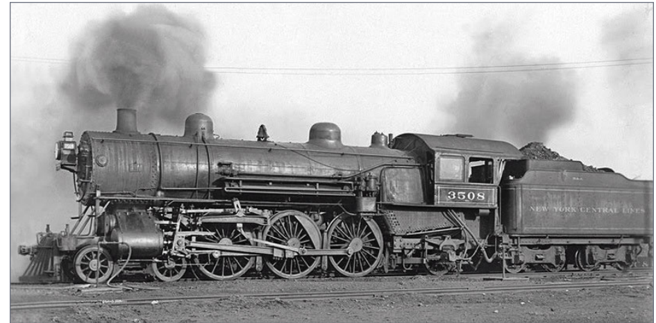
8. NYC Lines 4508 was assigned to the Boston & Albany to get its primary passenger trains over the mountains between Boston and Albany – where else?! It has clean lines, large drivers and the standard NYCL tender of the time. Note the old trucks under the tender. Photo circa 1905. Ray Breyer collection
