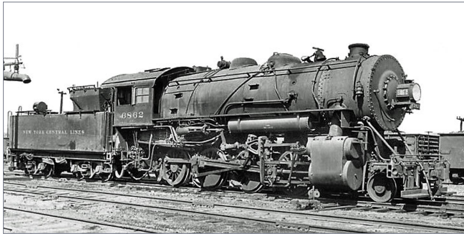
13. Here is another G5 2-8-0 parked alongside a water plug, circa 1930. The 6862 is NYC Lines, I suspect a Big Four locomotive. The G5 locomotives were large, hulky Consolidations. The tender is a switching tender that holds lots of water and little coal, and provides the crew with good rearward visibility.
