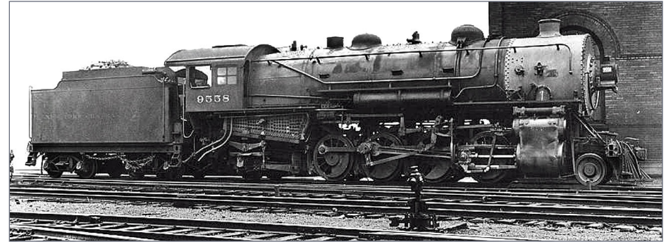
17. NYC Lines 9558 is an early H5 Mike rebuilt from a G5 class 2-8-0. Note that the small drivers were retained. It even has an early 2-8-0 small tender. Anyone modeling the NYC in the 1920-1950 time frame will need at least one of these locomotives. Photo circa 1925. Ray Breyer collection
