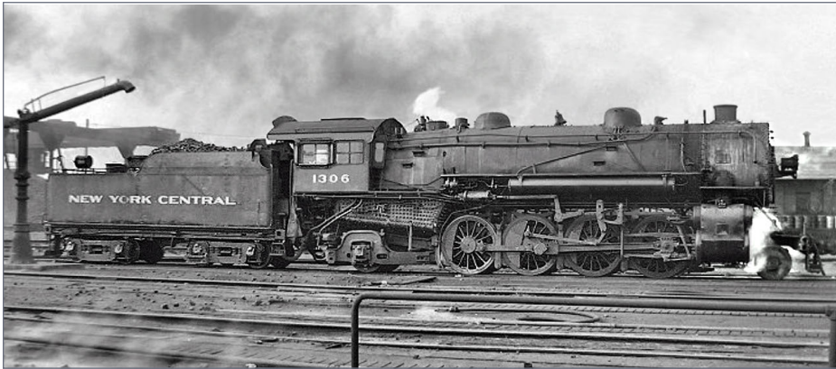
20. The 1306, a later-built H5, sits at the water plug in this photo from the 1940s. The white wisps of water vapor above the fire box and in front of the cylinders indicate this locomotive is under steam. Like the 6719 [18, 19], the 1306's tender is on passenger trucks. Ray Breyer collection
