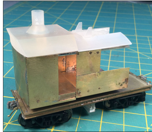
13. Here is the roof on top of the basic body. The cab walls were soldered together using a P-B-L resistance soldering unit.
