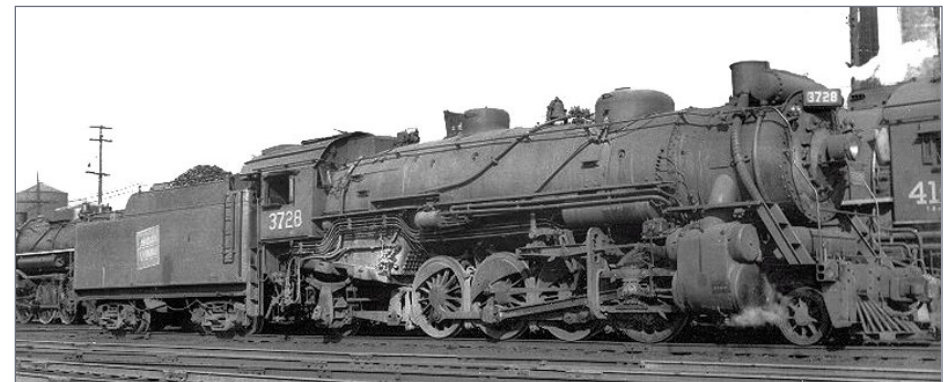
10. Very much appearing to be a USRA Mikado, this CN locomotive is one of 18 clones that the CN ordered. Note the Elesco feedwater heater atop the smokebox and the spoked pony truck wheel. Ray Breyer collection
