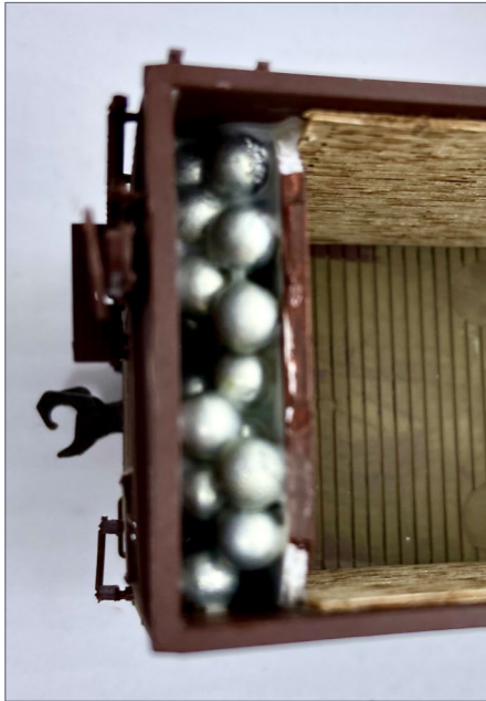
7. The bulkhead and shot installed on one end of the boxcar interior. I trimmed the top corners of the bulkhead so it does not interfere with the roof.
