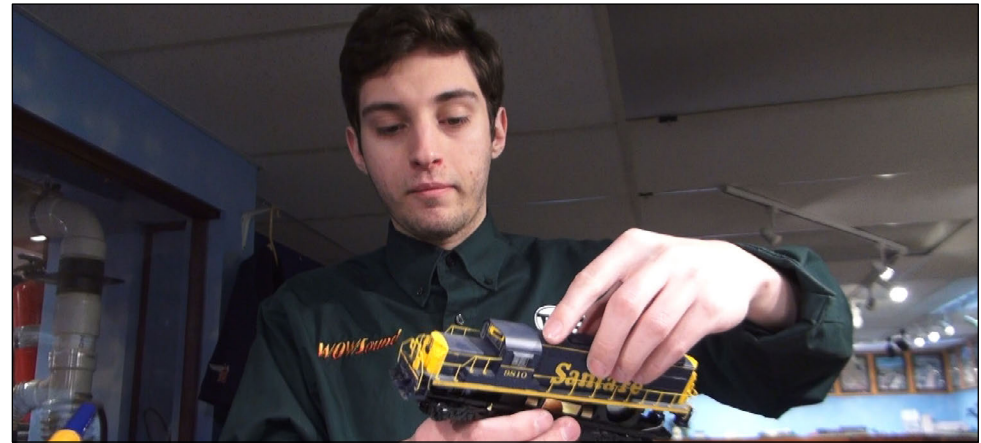
18. Here Dan reattaches the body shell and secures it by reinstalling the couplers.
