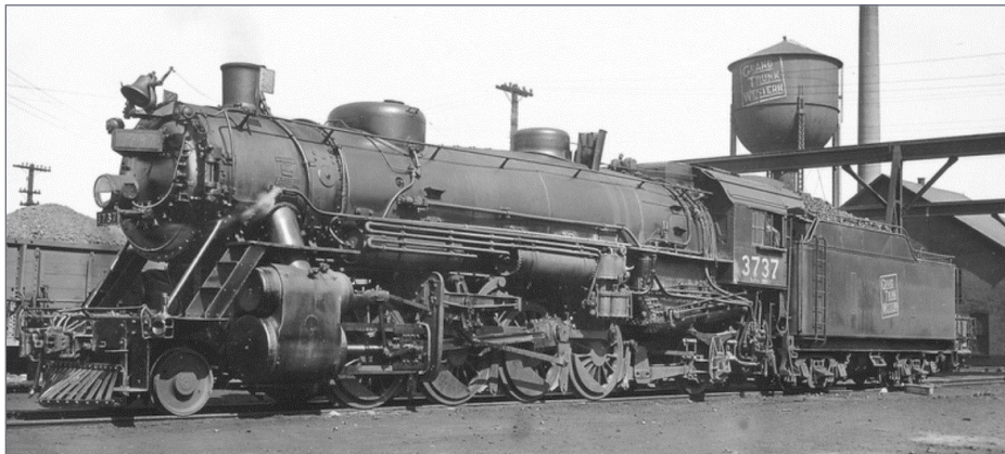
14. GTW 3737 Note the ladder up the side of the tender and the rerail frog between the tender trucks. Ray Breyer collection
