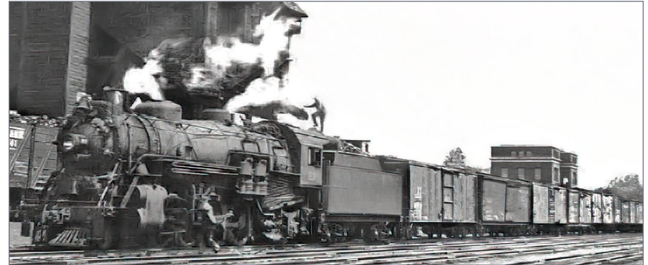
15. LH&HR #83 has a train of boxcars in tow. Note the two air pumps and the Worthington feedwater heater atop the smokebox between the bell and the smokestack. Also note the cow catcher front pilot. Ray Breyer collection
