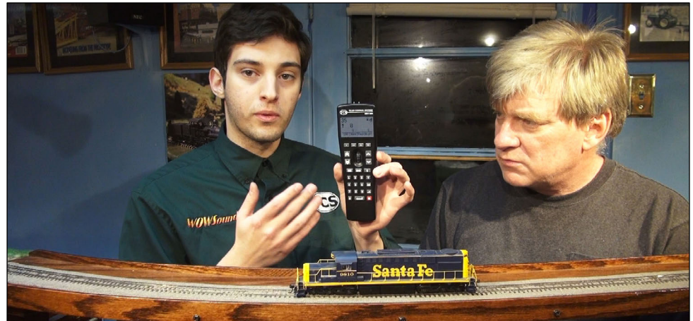
19. Dan completed the installation with a demonstration of TCS's Audio-Assist feature on the TCS WOWSound decoders, changing the horn and prime mover to the correct sounds by following Audio-Assist through a menu of options that he selected with Ken's TCS UWT-100. The UWT-100 was connected to Ken's Digitrax DCC system through a Digitrax LNWI (LocoNet WIFI Interface). See the video for a demonstration of how simple this is.
