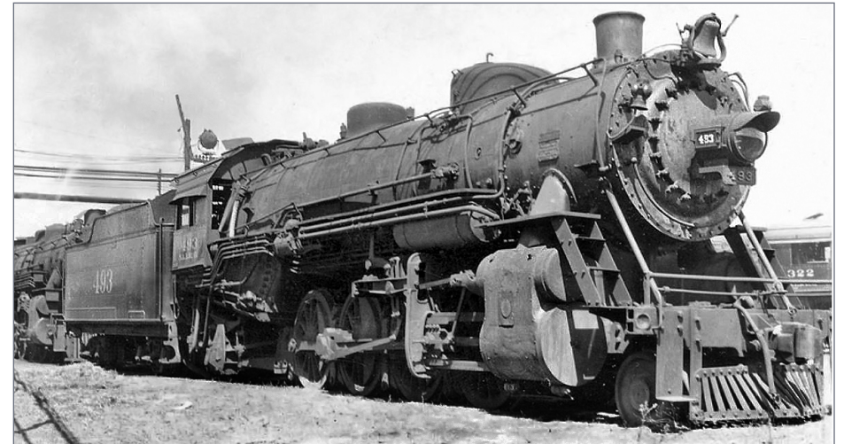
43. SAL 493 is shown ready to return to service on its next train. The locomotive has a cow catcher pilot with a small foot board at each side of the cow catcher. Plumbing from the sand dome has been re-installed in a slightly different arrangement. Ray Breyer collection
