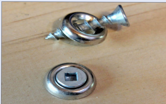
11. Flat-head screws and cup washers. No special reason for the square-drive screws – Phillips heads work as well.
