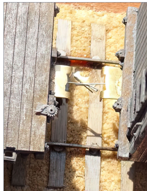
30. I formed the couplers from guitar string bent to shape in a jig. In UK practice, the car buffers maintain a distance when the vehicle is being propelled for uncoupling. I had to fashion a center buffer to represent the casting of the link-and-pin coupler, which is shown here still unpainted. To uncouple, a magnet or electromagnet buried in the track deflects the coupling downwards.
