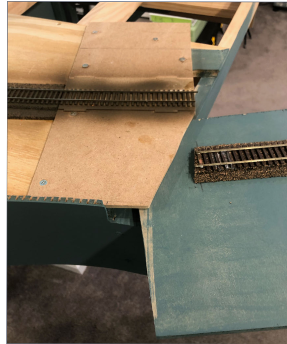
5. The gate in action! The end of the swing gate slides into the notch visible in photo 4. Note the paint scrapes indicating the friction lock. At some point we'll likely add an electrical interlock to kill power when the bridge is open.
