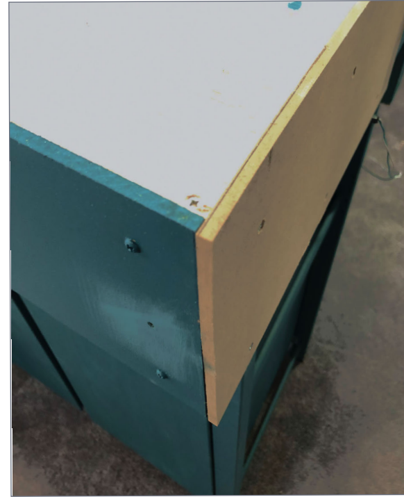
7. After catching my elbow on the sharp (ouch!) 90-degree fascia corners I opted to round the corners.
