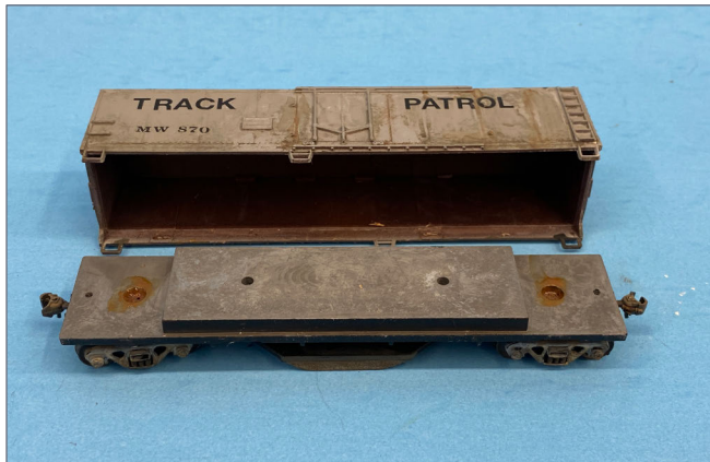
2. Lifting the shell off the Walther's car reveals a heavy metal floor.
