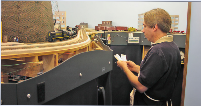
10. An op-session photo showing the bluish-green fascia, navy-blue drapes hiding under-layout storage, flat-head screws in cup washers (foreground), and miniature toggle switches installed on the 1/8"-thick fascia (background).
