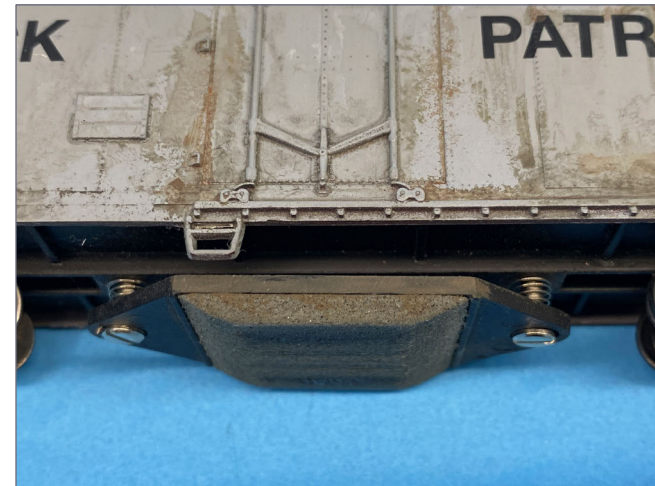
3. The cleaning pad assembly screws to the car, and a spring suspension helps press the cleaning pad to the rails.
