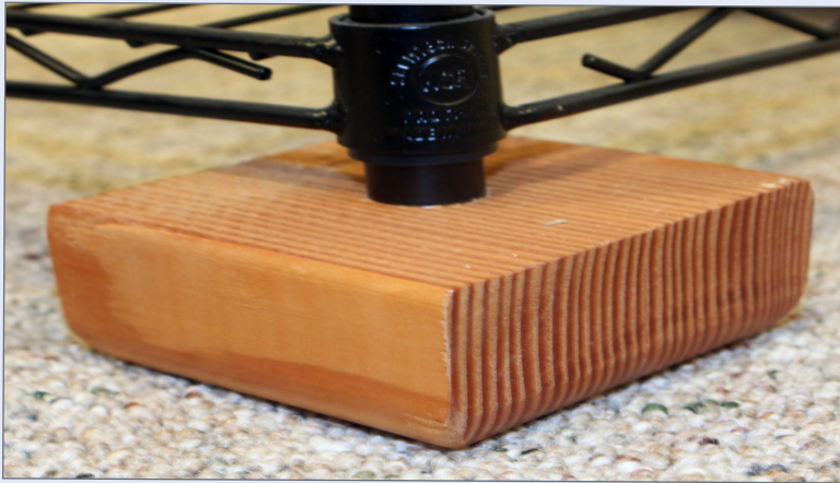
12. A foot made from 2x4 lumber. Each foot is 3-1/2" square, and the four bottom edges are rounded-over to 1/2" radius for easy sliding on carpet. The shelf leg fits into a hole drilled in the top.
