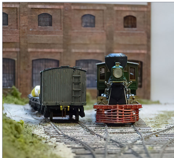
25. The view along the layout from the entrance to the staging yard shows the effect of the code 40 rail and broad gauge track. The siding on the left is laid with strap rail – flat metal strip laid directly on timber longitudinal bearers.
