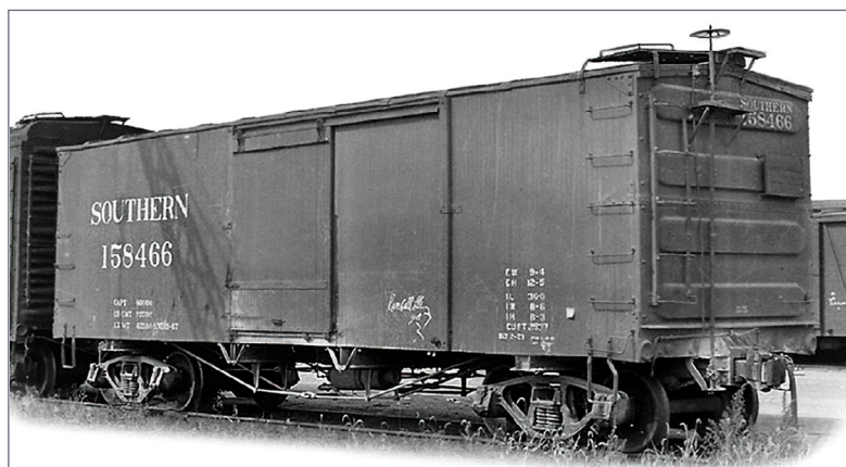
4. Southern 36-foot boxcar with stamped steel ends.
