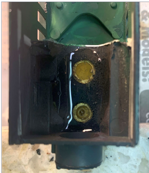
4. A pool of epoxy in the domes and the top of the boiler.
