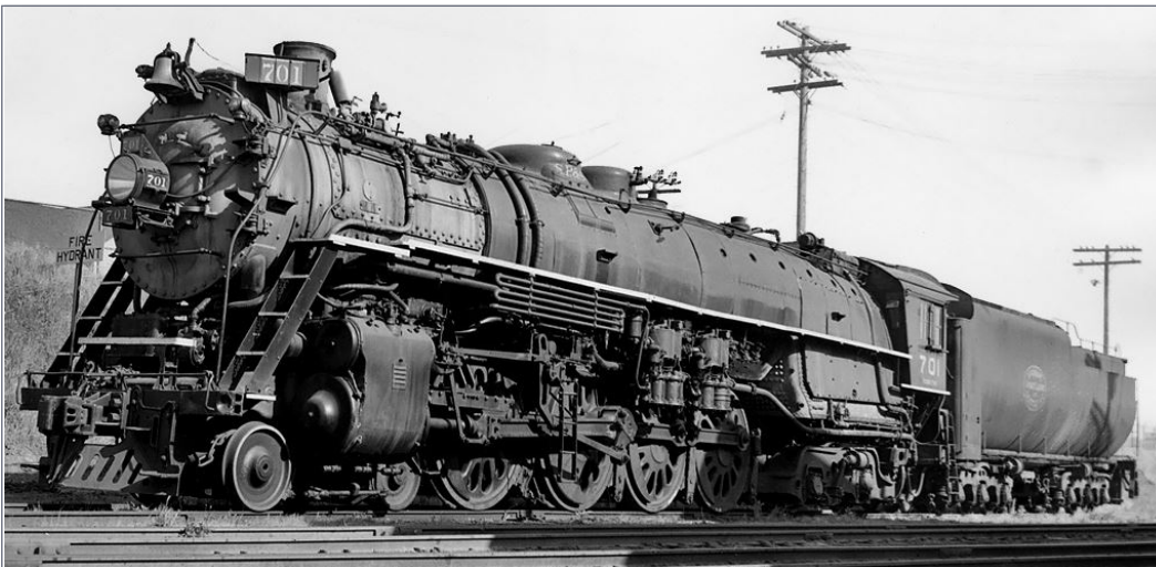
6. This is a nice profile view of SP&S 700. Clean, long, and powerful describe the appearance of this locomotive. Baldwin delivered the 700 to the SP&S on June 21, 1938. The three SP&S E1 class locomotives were oil-burners. Ray Breyer collection
