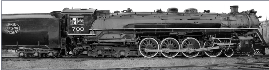
6. This is a nice profile view of SP&S 700. Clean, long, and powerful describe the appearance of this locomotive. Baldwin delivered the 700 to the SP&S on June 21, 1938. The three SP&S E1 class locomotives were oil-burners. Ray Breyer collection
