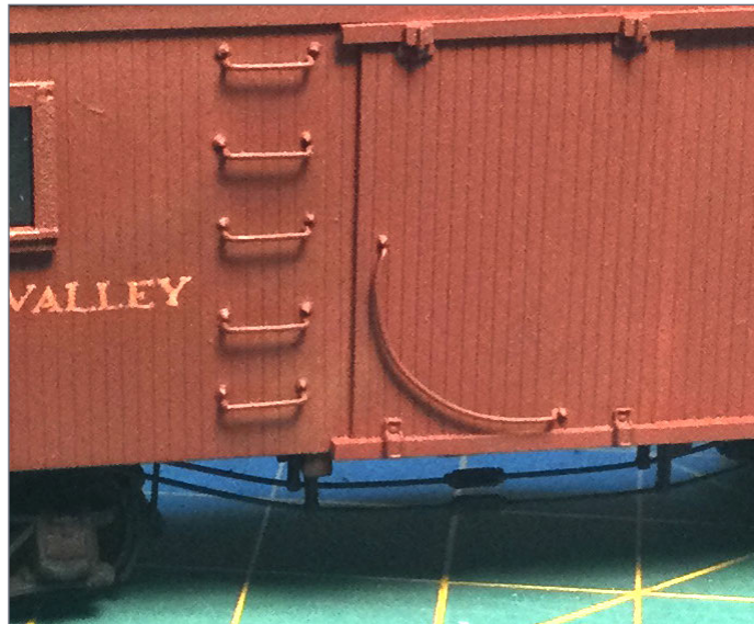
9. One of the six curved grab irons on two cabooses.
