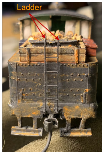
3. This separately applied ladder from Grandt Line looks much better than the molded-on ladder. Note the modifications I made to the pilot steps as compared to [1].
