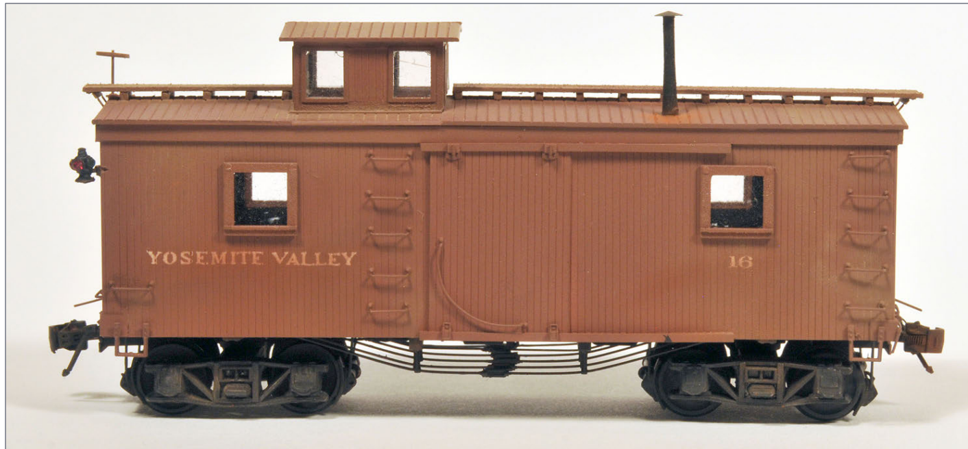
16. The second caboose No. 16 with the curved roof and a cupola which was narrower than the roof.
