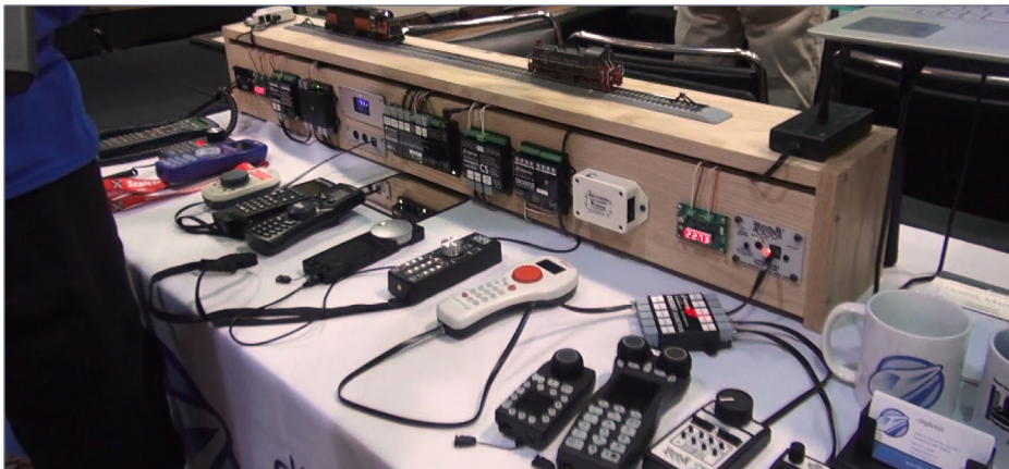
15. The Digikeijs DR-5000 supports throttles and accessories from many different manufacturers, as well as having built-in WIFI support. See the June 2019 issue ( model-railroad-hobbyist.com/magazine/mrh2019-06/dr5000 ) of MRH for a First Look article on the DR-5000 command station.
