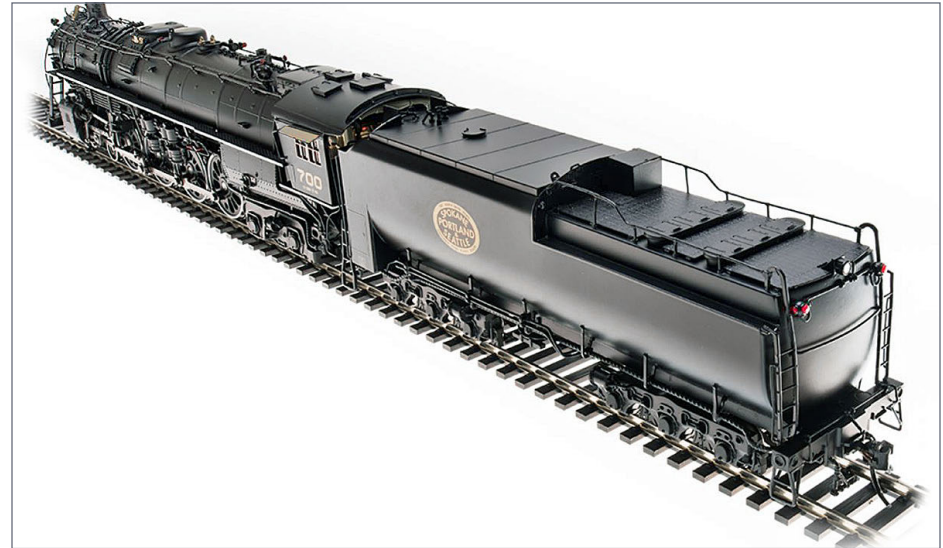
12. Broadway SP&S 700 shows the tender fitted with an oil tender matching the oil-burning Spokane Portland & Seattle E1-class locomotives. Broadway Limited Imports photo
