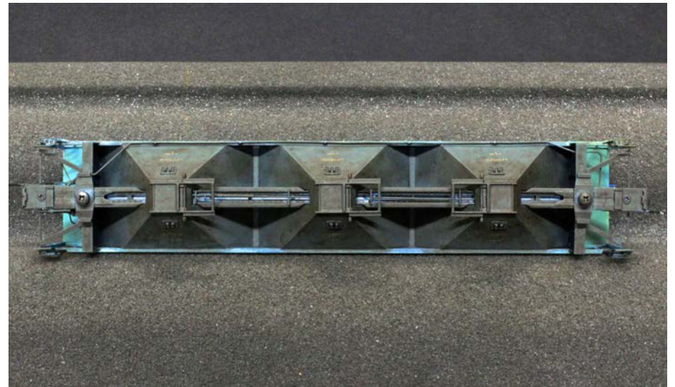
18. I applied a layer of dark brown, almost black grime to the bottom of the car. I used a series of highly thinned acrylic paint washes of burnt umber and black to achieve the effect.
