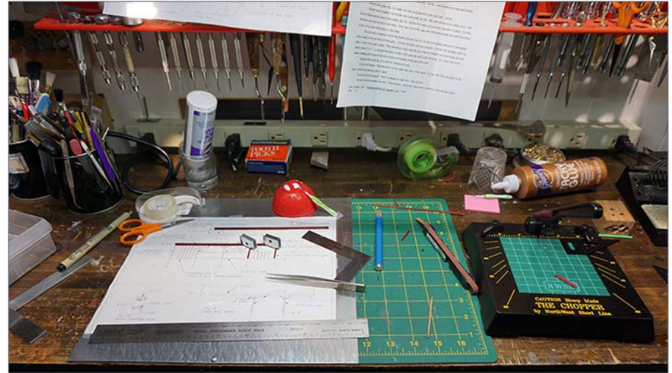
17. My workbench with the magnetic assembly jig. The drawings and a layer of mylar are on top of the steel plate to begin frame assembly. The plans hang from a pegboard to save desktop space.
