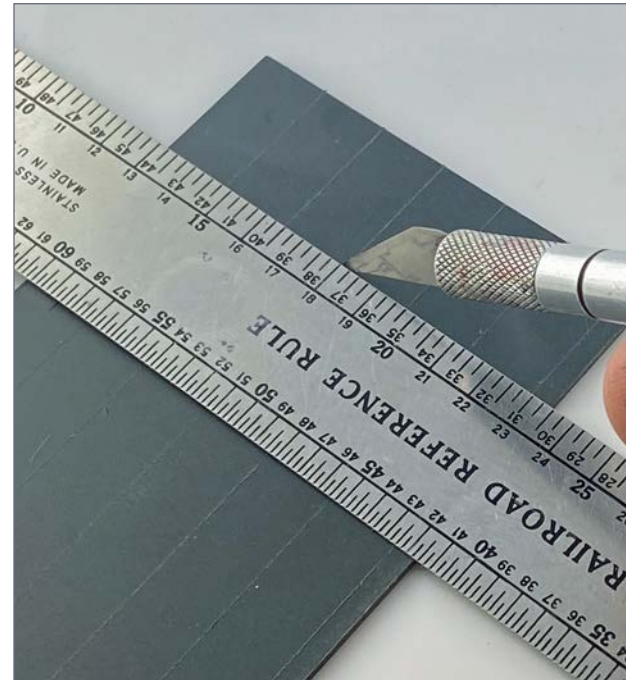
23. Most rolls are around 100' long, so I measure along the horizontal and scribe seams to represent the transition from one roll to the next. Then I dust the roof with flat black spray paint. As with the sloped roof, the aim is for a spattered look.
