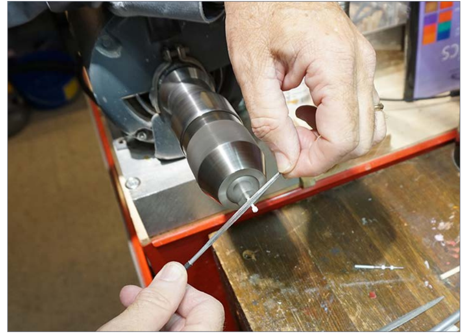
11. I acquired my bench motor during my flute-making days. With a 1725 rpm spin rate, a high-end chuck, hollow shaft, and custom hand brake, it functions as my “poor man’s lathe.”
