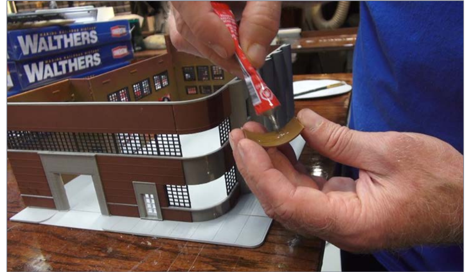
10. Ken puts glue onto the backs of the curved brick inserts and then simply places them into the walls.
