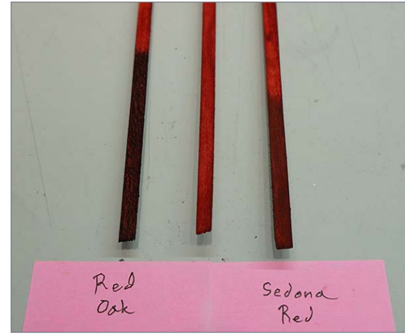
13. The center strip is the unsatisfactory red. The Red Oak stain was too dark. The Sedona Red looked best, though I applied it too heavily in this photo.
