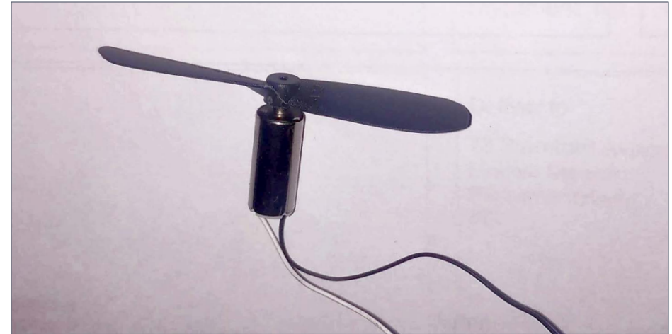
2. Electric drone motor and propeller.
