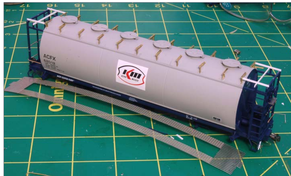
3. Applying the Plano photo etched roof walk.
