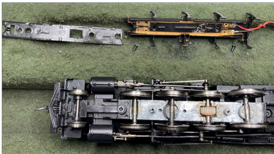
6. Axle cover plate removed.
