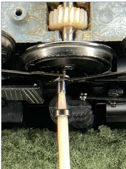
16. Using a toothpick aided proper reassembly.
