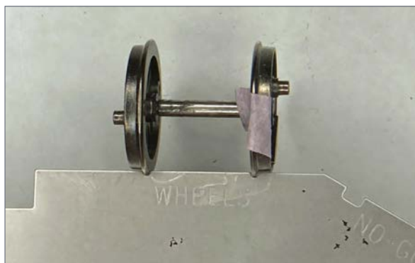
14. The wheel is properly quartered and gauged.
