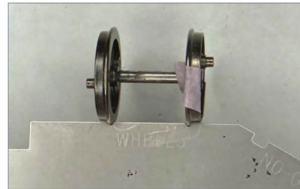
14. The wheel is properly quartered and gauged.
