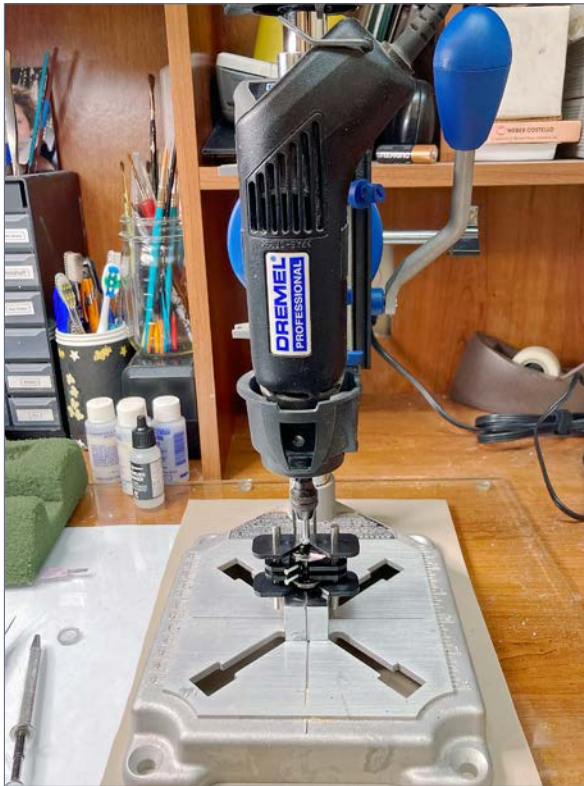
13. Using my Dremel Workstation to press the quartered wheel back onto the axle.
