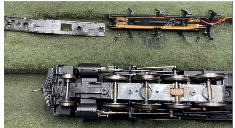
6. Axle cover plate removed.
