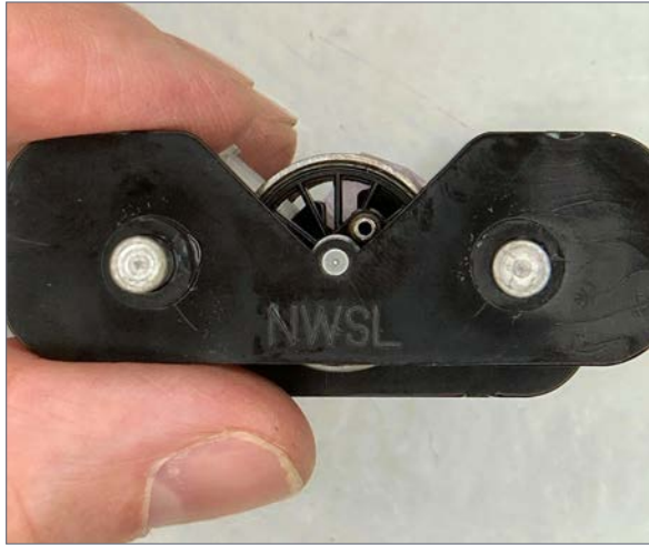
10. The engineer's side driver attachment point is in place in The Quarterer.
