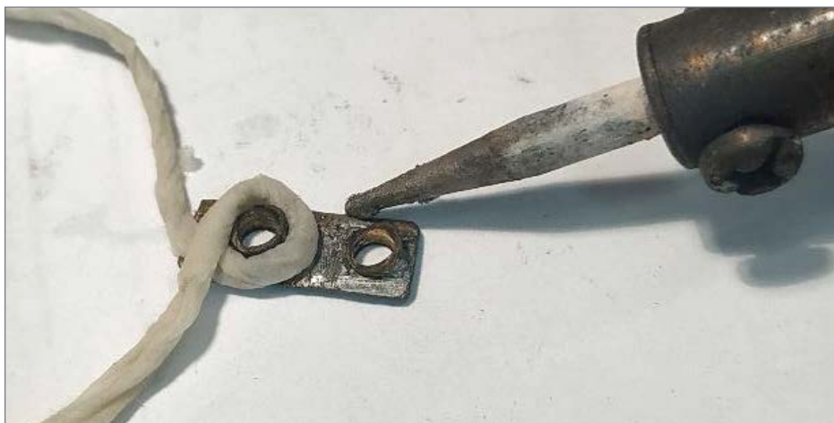
5. Soldering the second signal hood onto the head.
