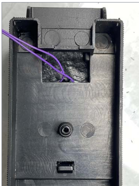
19. The wires extend into the tender shell from the coal load.
