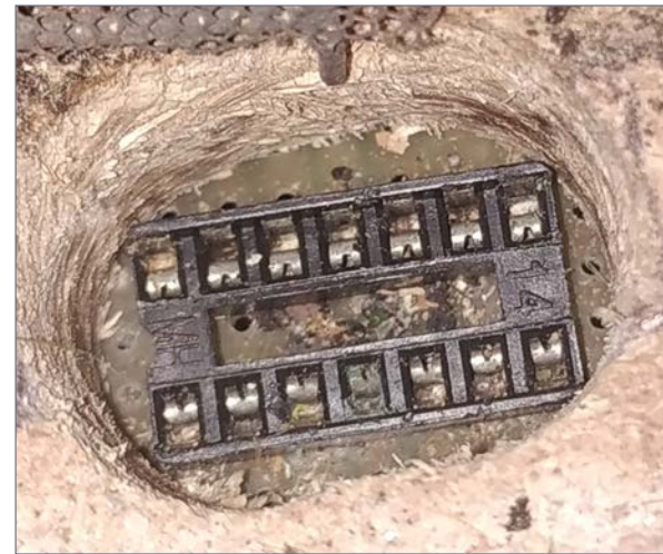
12. This DIP socket is at the right height in the layout. This socket has 14 pins instead of eight. This basic design for bump-resistant signals can be expanded to accommodate a variety of signals.
