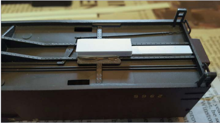
7. The 1/8 x 1/4-inch block is in place. Note the spacing between the block and the end of the car is sufficient for Kadee #451 swing-arm draft gear.
