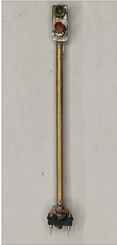
11. The completed signal is ready for paint.
