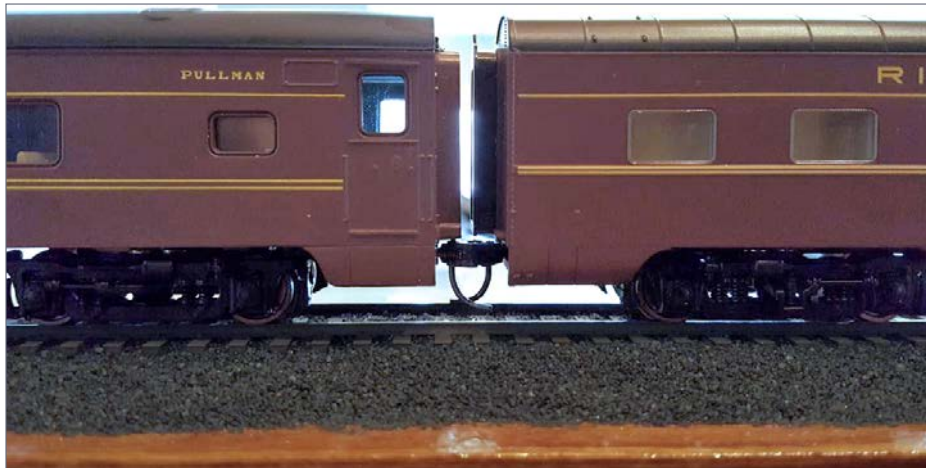
13. This is a converted Rivarossi tail car (on the left) coupled to a Walther's passenger car to verify car and coupler height and compatibility.
