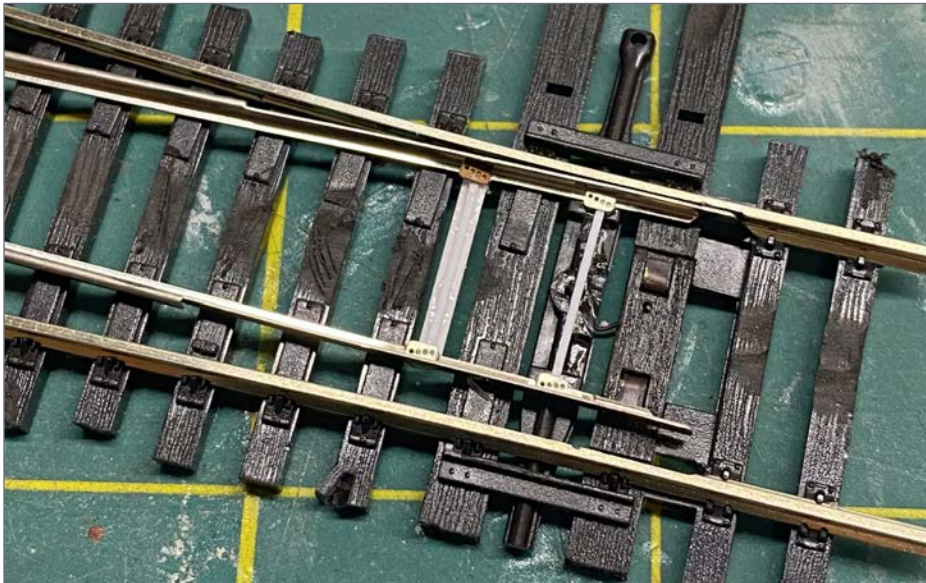
6. The hinge details are in place.
