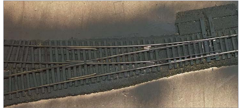
11. The turnout was sprayed camouflage brown.
