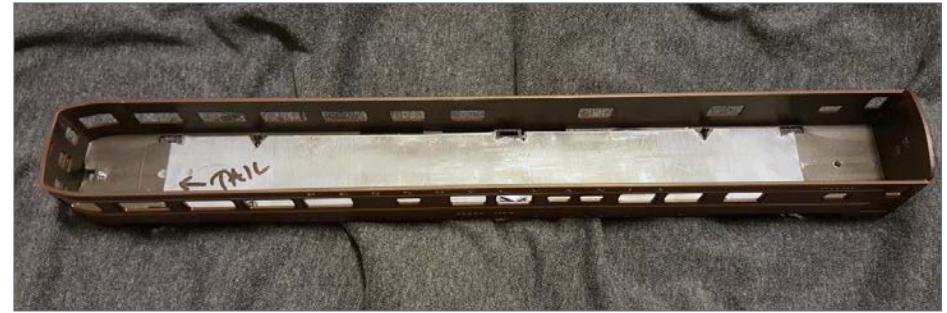
14. This is the "tail car" with the sheet of the LSW118 lead before I glued it into the car. Notice that I snipped around the various protrusions so the sheet would lie flat. I have since determined that a hand-held hole-punch does a much better job of making the notches.
