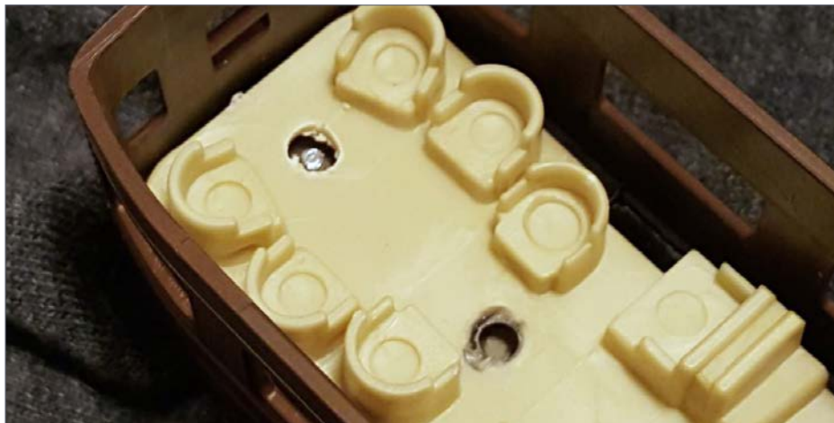
16. The holes are ugly, but necessary to clear the screws.
