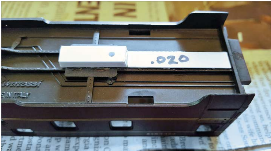
8. The mounting hole is drilled. I found that the Kadee mounting area needed a 0.020" shim to fit flush with the end of the car.
