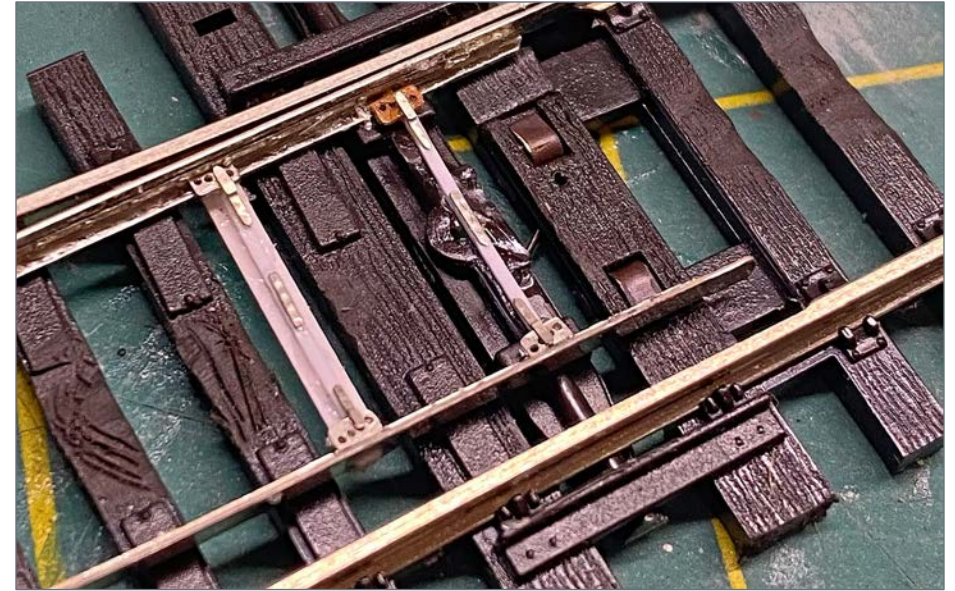
7. The throw rod detailing was the final step. Gluing fine, photo-etched metal details to a 0.010" styrene surface was a challenge. I recommend a set of very small tweezers and some patience during this step.
