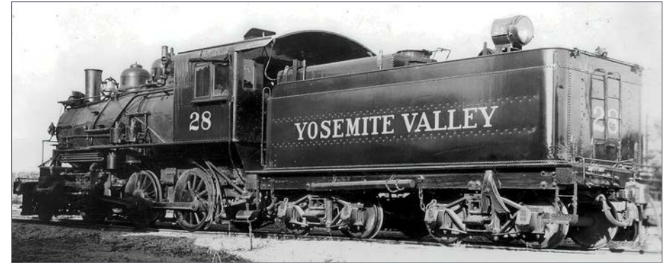
19. This photo of the No. 28 shows the air hose for the side dumps to the left of the rear coupler. Larry Harrison photo
