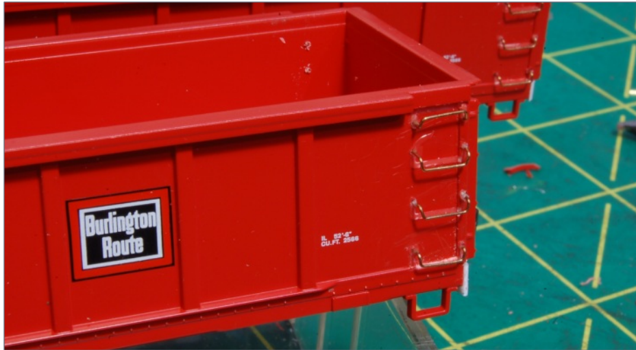
3. The newly installed wire grab irons look good.
