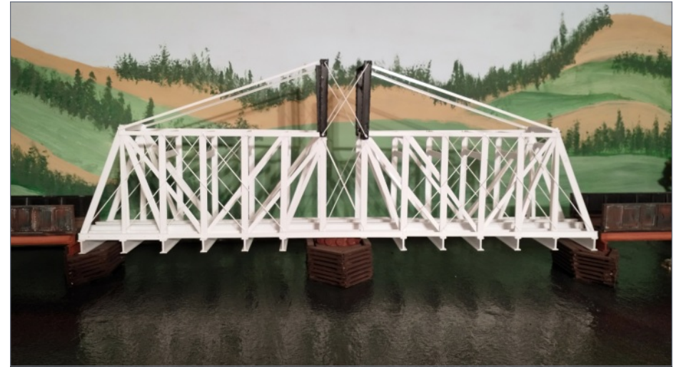
15. I used 2.4mm angle for the span braces across the top of the bridge for extra strength. I added cross wires to the center portion of the superstructure.
