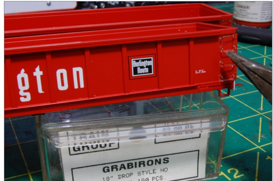
2. I put the grabs in place with needle-nose pliers. The “shadows” from the cast-on grab irons made it easy to place the mounting holes.
