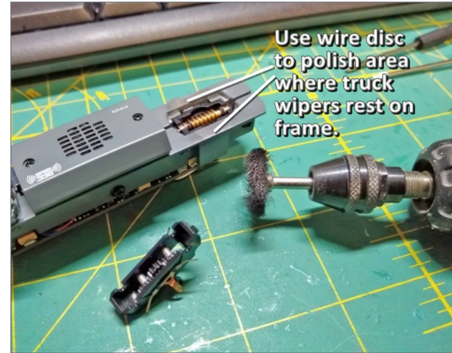
13. I dismantled the truck and cleaned all the parts. I also polished the frame where the truck wipers make contact.
