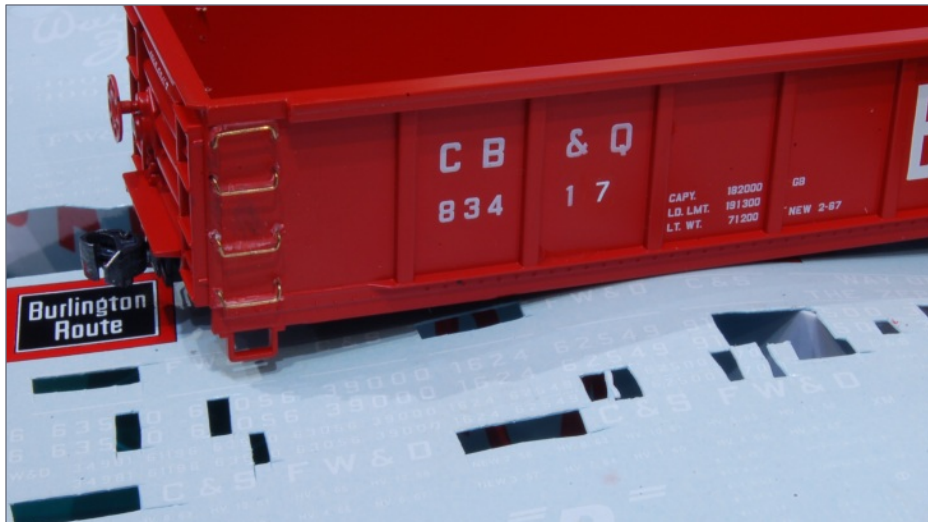
4. Although I found all three cars on the Rail Pictures Archive website, I decided that the photo for 83417 – not among my models – was more inspiring because it was still wearing the ACI label. I scraped off the final digit on my 83416 with a no. 11 blade and replaced it with a “7” from a MicroScale CB&Q boxcar set.
