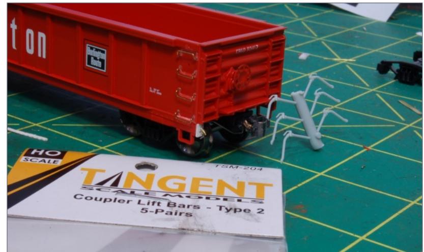
6. Although I have bent hundreds of coupler cut levers from 0.012” brass wire, I found Tangent makes the appropriate cut lever (TSM 204). This was much more convenient, especially since I was doing three cars!
