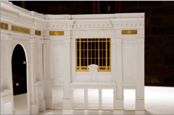
29. The styrene and brass master pattern for the grand lobby's end walls.
