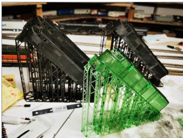
14. My resin 3D-printed shells, freshly washed and cured.
