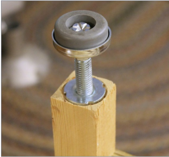
4. Elevator bolts in each leg allow adjusting the height and leveling the layout.
