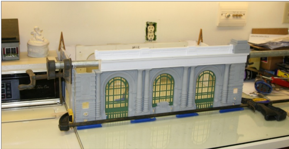
3. Furniture clamps hold the pieces together as the head house is assembled. Styrene masters for the entablature and pediment can be seen under construction in white.
