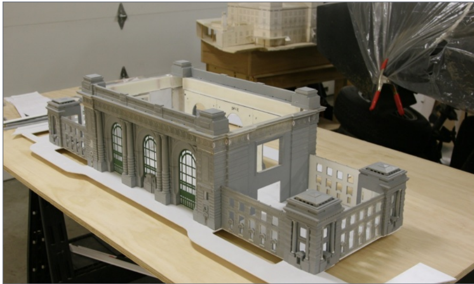
11. The front and rear pediments and entablature pieces as well as the columns for the end towers have been cast and installed.
