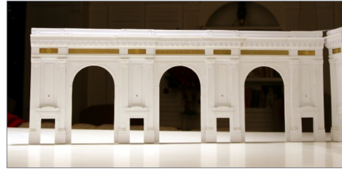
28. The styrene and brass master pattern for the grand lobby's side walls.
