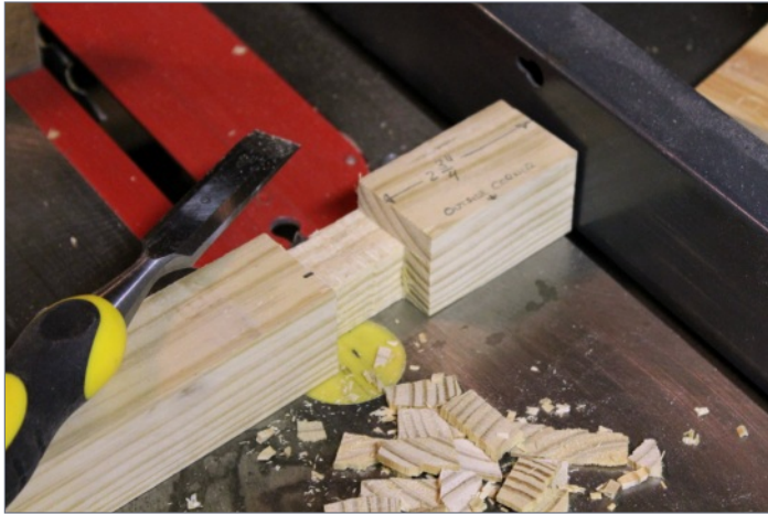
7. Finished pair of slots in the leg, ready for assembly of the box skeleton.
