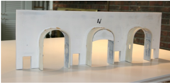
32. The “arch liner” pieces have been cast-formed and glued in place to the inside wall.
