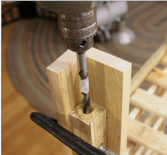
5. Drilling the holes for the elevator bolts.
