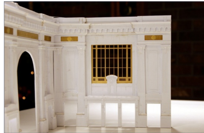
29. The styrene and brass master pattern for the grand lobby's end walls.
