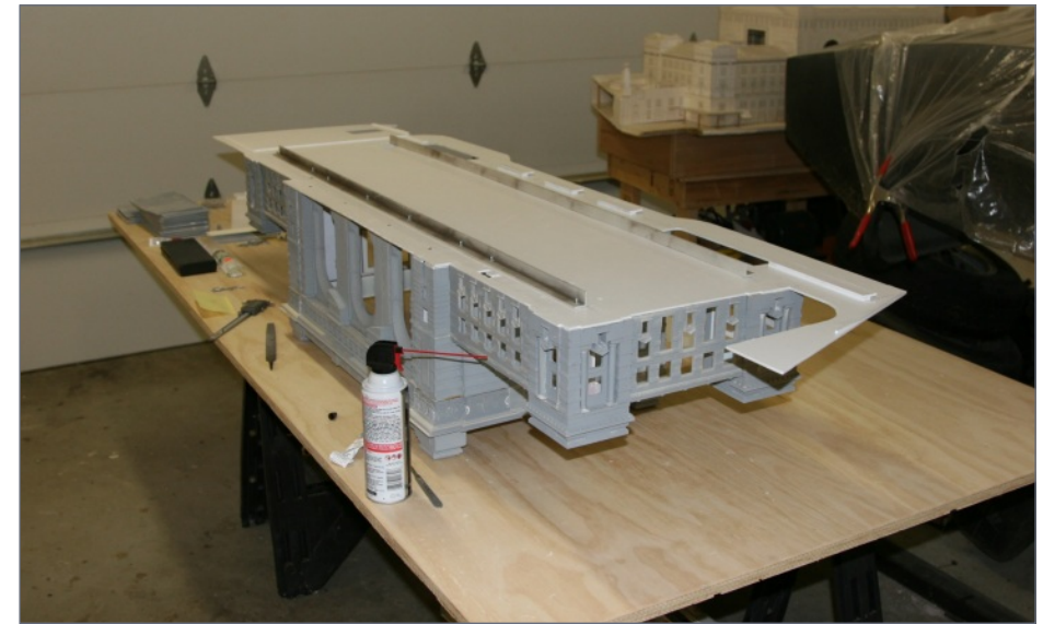
12. I bolted aluminum angle braces on to stiffen the base. The original foam core mockup is in the background.
