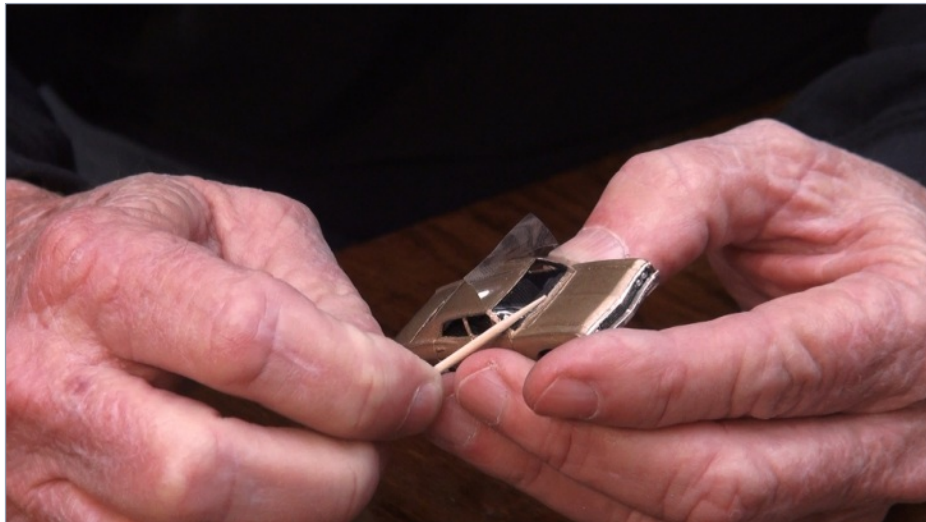
17. Mike burnishes the tape into place.
