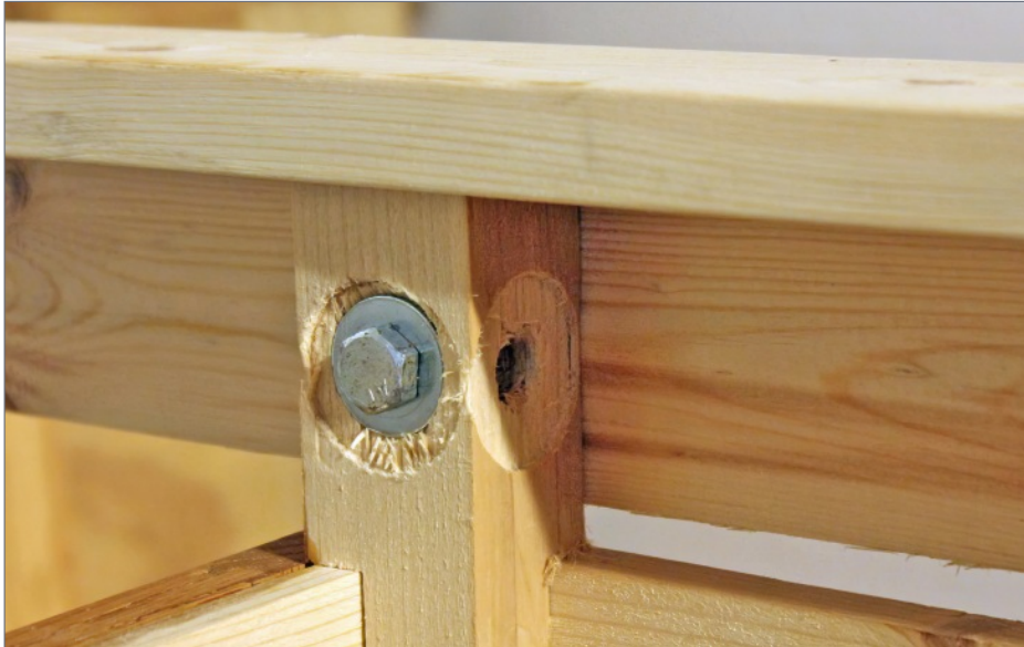
3. Holes in the leg top for connecting the benchwork box to the layout L-girders.
