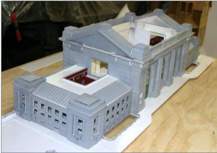
21. I built the sloped roof portions at each end from styrene and covered them with cast roofing material.
