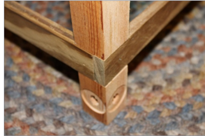
8. Overlapping joint at each leg. Glue the stretchers into the slots in the leg and secure them with a finishing nail.
